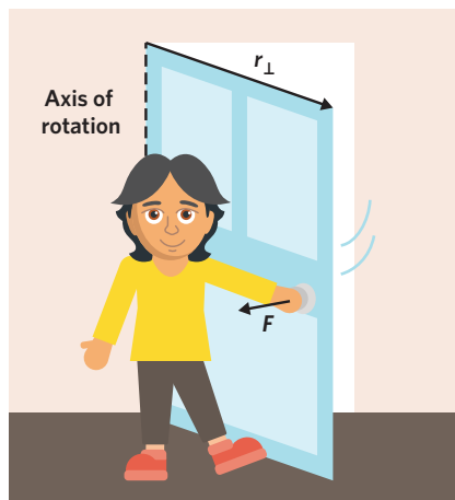
Figure 2 Applying a torque to a door
