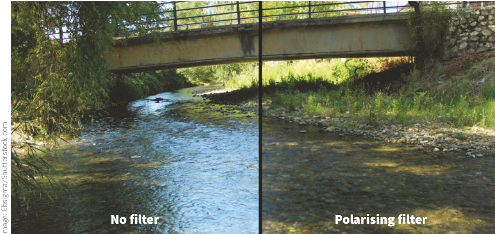
Figure 2 A comparison of viewing the surface of water without (left) and with (right) a polarising filter. The filter blocks the reflections from the water, which were polarised in a different direction to the filter.
