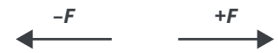
Figure 1 Force vectors with magnitude F in the negative (left) and positive (right) directions. Here the positive direction has been defined as to the right.
