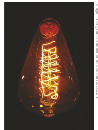
Figure 4 The heated tungsten filament of an incandescent globe
