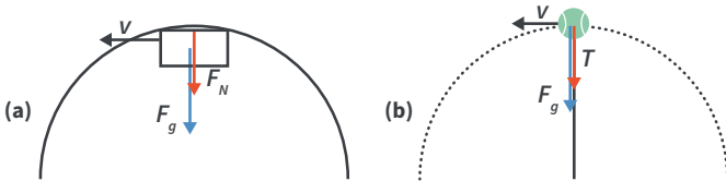
Figure 2 (a) An object moving on the top and inside of a vertical circle. (b) This is equivalent to a ball on a string at the top of its vertical circular motion.
