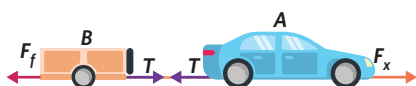
Figure 1 The horizontal forces involved for car, A, which is towing a trailer, B
