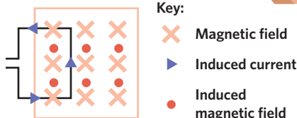
Figure 4 Right-hand coil rule applied to a loop entering a magnetic field
