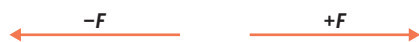
Figure 1 Force vectors with magnitude F in the negative (left) and positive (right) directions. Here the positive direction has been defined as to the right.
