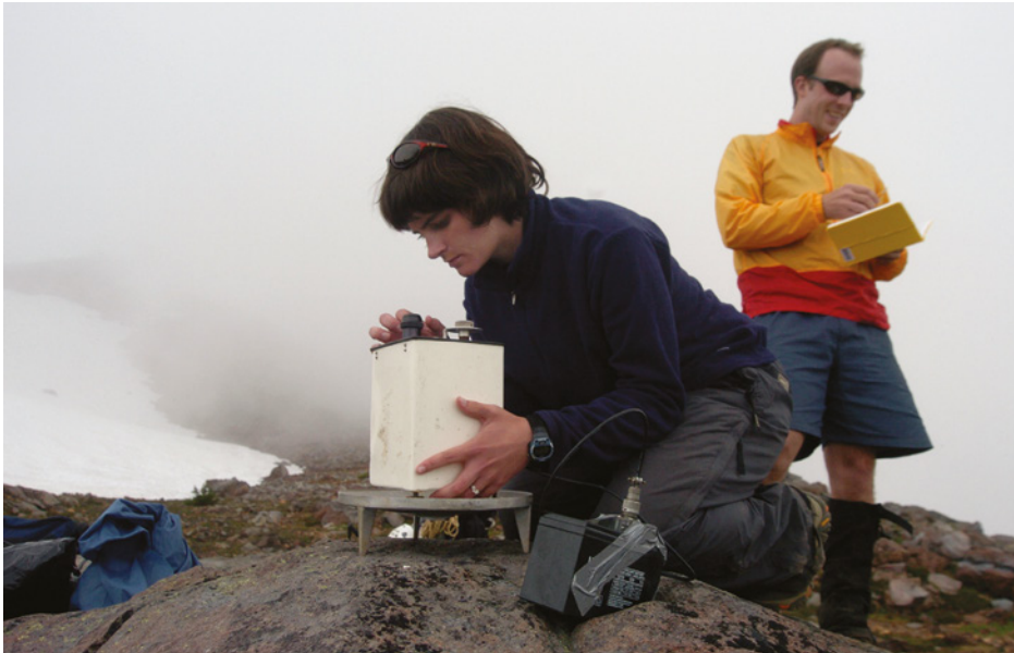
FIGURE 1.2.6 A gravimeter can be used to measure the strength of the local gravitational field.
