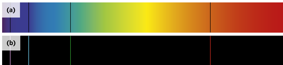
FIGURE 10.3.5 In the absorption spectrum of hydrogen (a) there is a background of continuous white light (broken into a spectrum of colours), with black lines that correspond to wavelengths of the radiation absorbed by the hydrogen atoms. In the emission spectrum of hydrogen (b) there is a black background against which lines corresponding to the wavelengths emitted by the hydrogen atoms can be observed.
