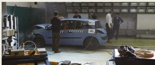
FIGURE 7.1.7 The Australian New Car Assessment Program (ANCAP) assesses the crashworthiness of new cars. This car has just crashed at 50 \text{ km h}^{-1} into a 5-tonne concrete block. The crumpling effect can clearly be seen.
