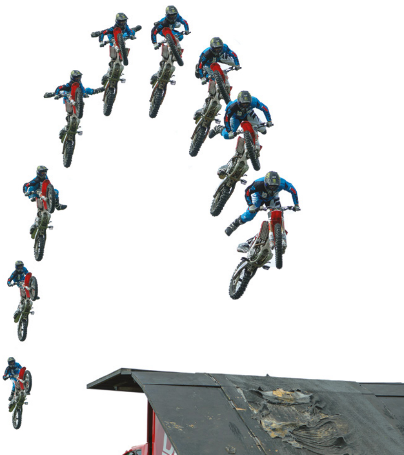
FIGURE 5.5.2 The motorcycle and rider are travelling in parabolic paths as they fly through the air.
