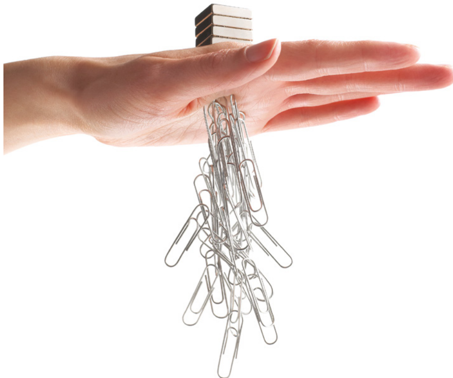
FIGURE 2.5.1 The magnet has an effect on the paper clips even though they are not in contact. This is because the paper clips are within the magnetic field produced by the magnet.
