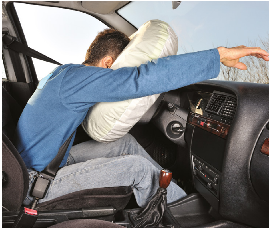
FIGURE 7.1.4 Airbags reduce the force on passengers by extending the time that it takes for them to stop.
