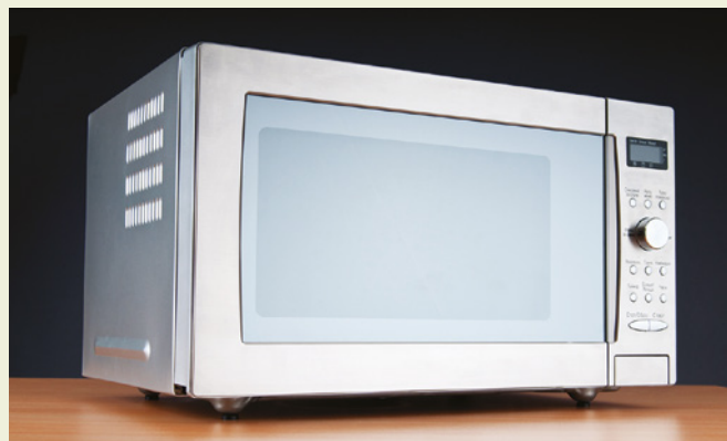
FIGURE 9.3.5 Microwave ovens produce electromagnetic radiation with a frequency of 2.45 GHz, which is the resonant frequency of water molecules.
