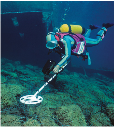
FIGURE 4.3.1 A diver using a metal detector. If a metal object is found underneath the coil of the detector, an emf will be induced which creates a current that will affect the original current. The direction of the induced current is predicted by using Lenz's law.
