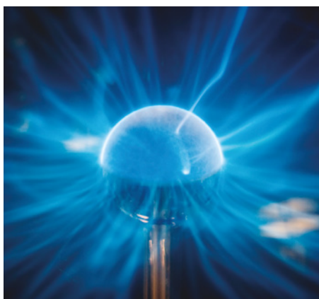
FIGURE 2.1.1 Charged plasma follows lines of the electric field produced by a Van de Graaff generator.
