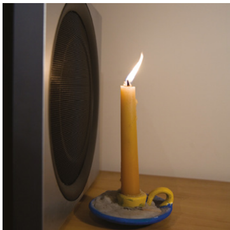
FIGURE 8.1.5 The motion of a flame in front of a loudspeaker is clear evidence of the continuous movement of air backwards and forwards as the loudspeaker creates a sound wave.
