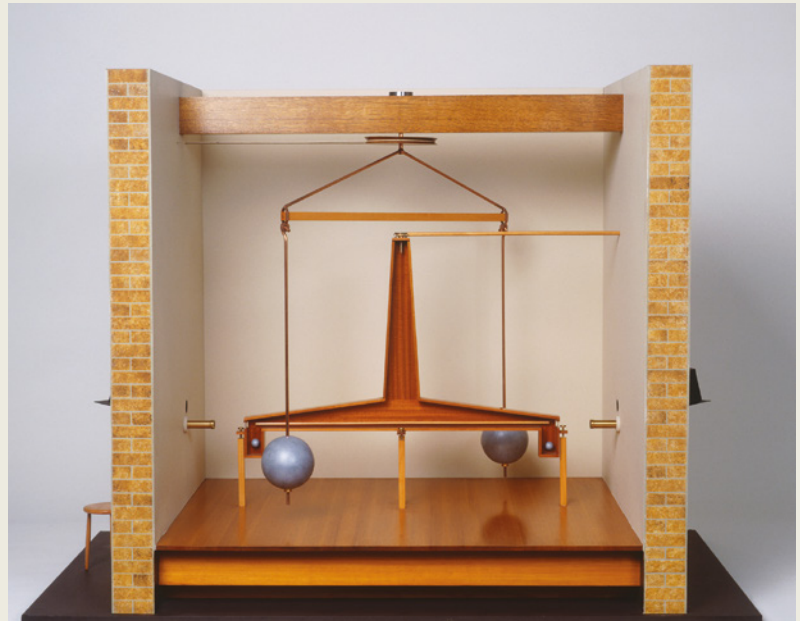
FIGURE 1.1.3 Henry Cavendish used a torsion balance to measure the small twisting force created by the gravitational attraction of lead balls.
