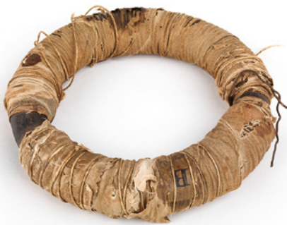
FIGURE 4.1.1 Michael Faraday's original induction coil. Passing a current through one coil induces a voltage in the second coil by a process called mutual inductance. This coil is now on display at the Royal Institution in London.
