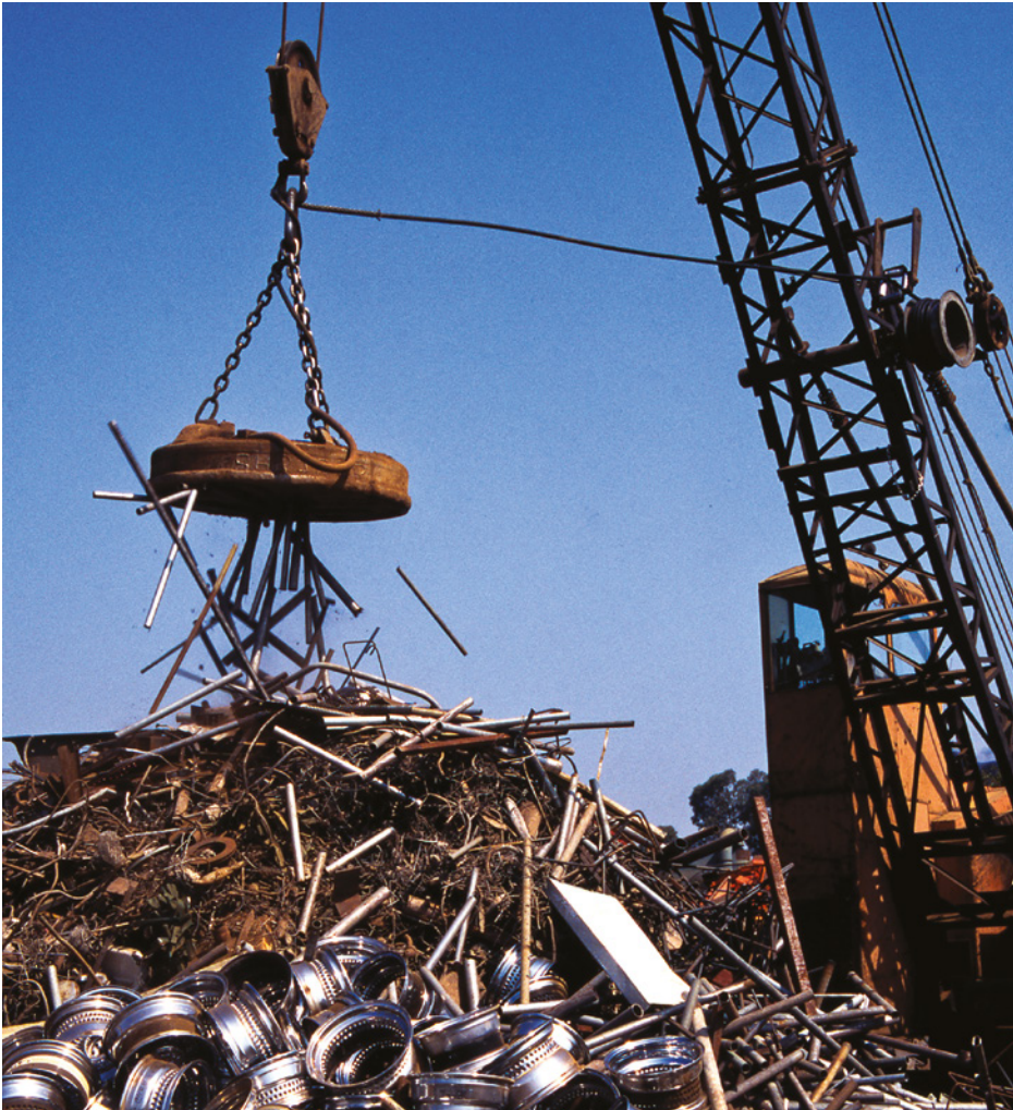
FIGURE 2.3.18 A large electromagnet being used to lift waste iron and steel at a scrapyards. Valuable metals such as these are separated and then recycled.
