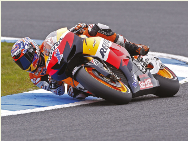
FIGURE 5.3.7 Australia's Casey Stoner won the 2012 Moto GP championship. Here he is leaning his bike as he takes a corner at Phillip Island. Leaning into the corner enables him to corner at higher speeds. In fact, the bike would go out of control if he did not lean it.
