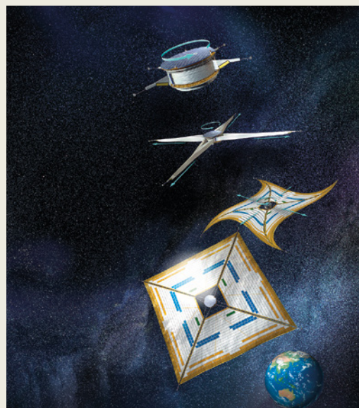
FIGURE 10.2.10 The IKAROS spacecraft is the first interplanetary spacecraft to use solar-sail technology.
