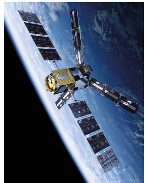
FIGURE 3.1.14 A low-orbit satellite called the Soil Moisture and Ocean Salinity (SMOS) probe was launched in August 2014. Its role is to measure water movements and salinity levels on Earth as a way of monitoring climate change. It was launched from northern Russia by the European Space Agency (ESA).
