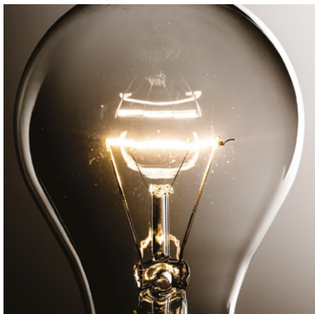
FIGURE 10.3.12 In an incandescent light globe, electricity is passed through a tungsten filament. As the filament heats up, the free electrons in the tungsten atoms collide, accelerate and emit photons. A wide range of photon wavelengths are emitted due to a wide range of different collisions (some weak, some strong).
