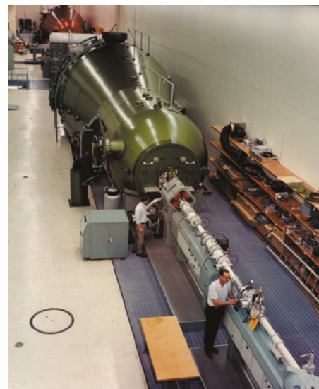
FIGURE 3.3.2 This tandem Van de Graaff accelerator uses two generators to produce beams of charged particles that are accelerated by potential differences of up to 10 million volts.
