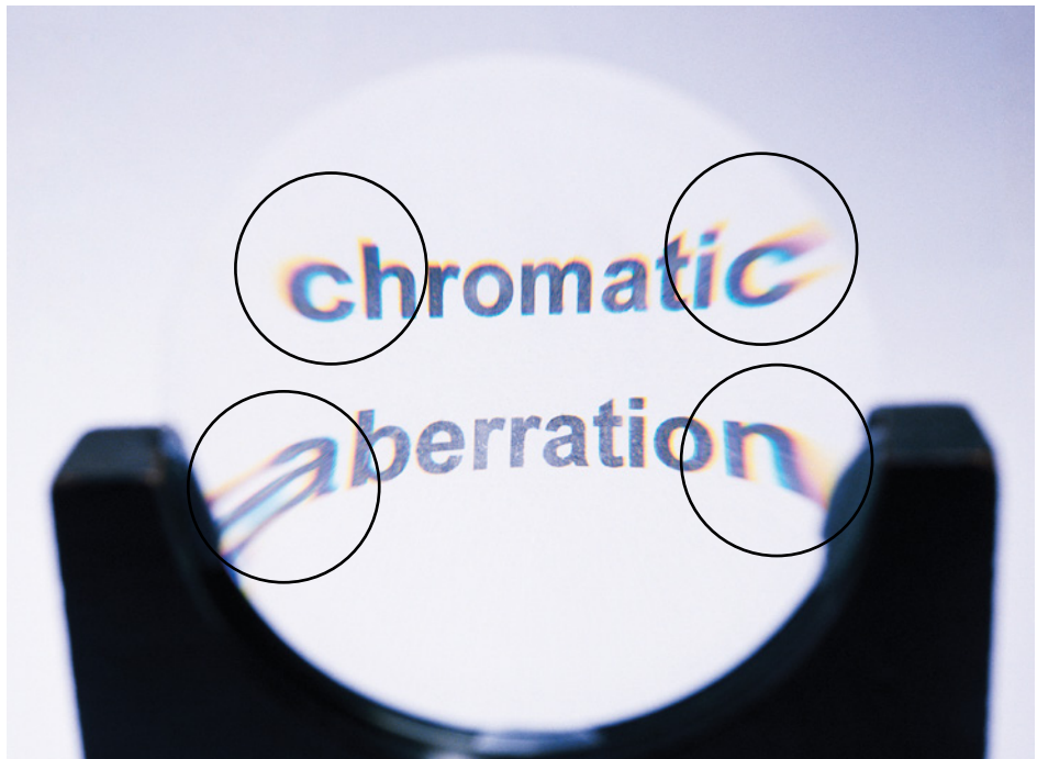
FIGURE 9.1.14 Chromatic aberration causes the coloured fringes that can be seen in the circled regions in this image.
