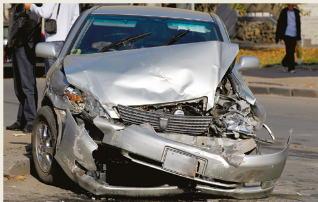
FIGURE 7.1.6 Cars are designed with weak points in their chassis at the front and rear that enable them to crumple in the event of a collision. This extends the time over which the cars come to rest and so reduces the size of the forces acting on the occupants.
