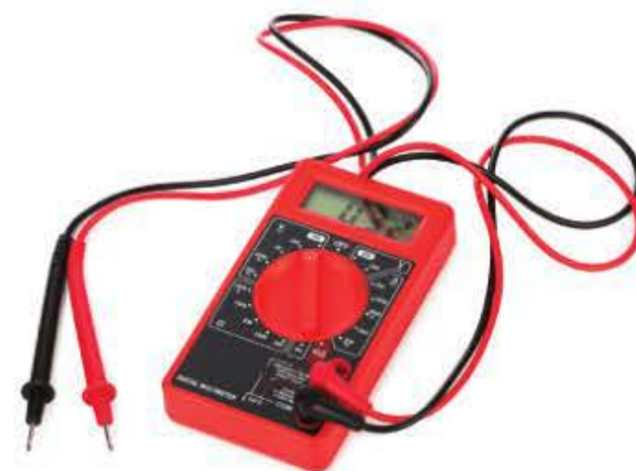
FIGURE 8.3.5 A digital multimeter can be used as either an ammeter or a voltmeter.
