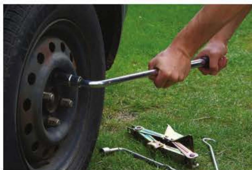
FIGURE 14.1.10 Removing a tyre with an extended handle spanner will increase the torque on the nut.
