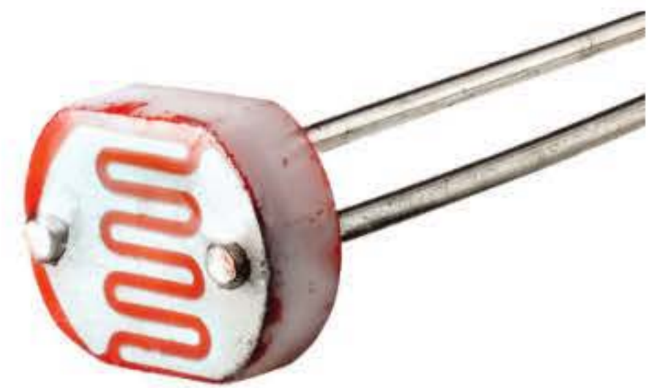
FIGURE 9.2.7 The resistance of a light dependent resistor changes depending on how much light is falling on it.
