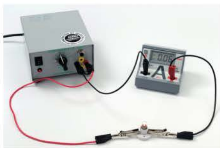
FIGURE 8.2.7 A digital ammeter (labelled with an A) measures current in a circuit.
