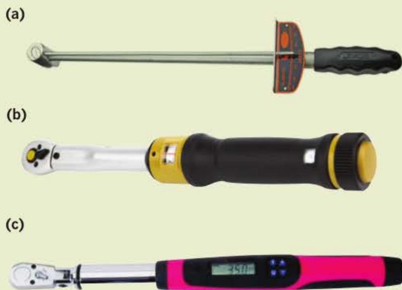
FIGURE 14.1.15 Three types of wrenches commonly used to measure the torque applied to a nut or bolt: (a) beam torque wrench, (b) a click-type torque wrench, and (c) an electronic torque wrench
