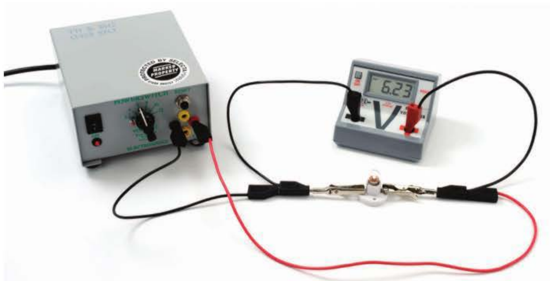
FIGURE 8.3.4 A voltmeter measures the voltage change (in this case, 6.23 V) across a light bulb.
