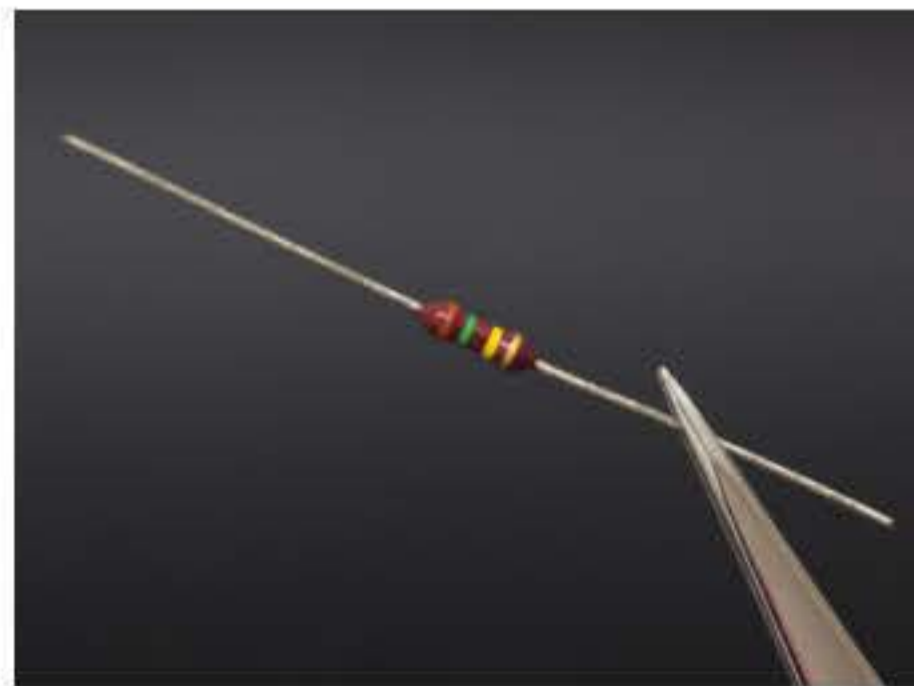
FIGURE 8.4.4 Common resistors are electrical devices with a known resistance. The coloured bands indicate the resistor's resistance and tolerance.
