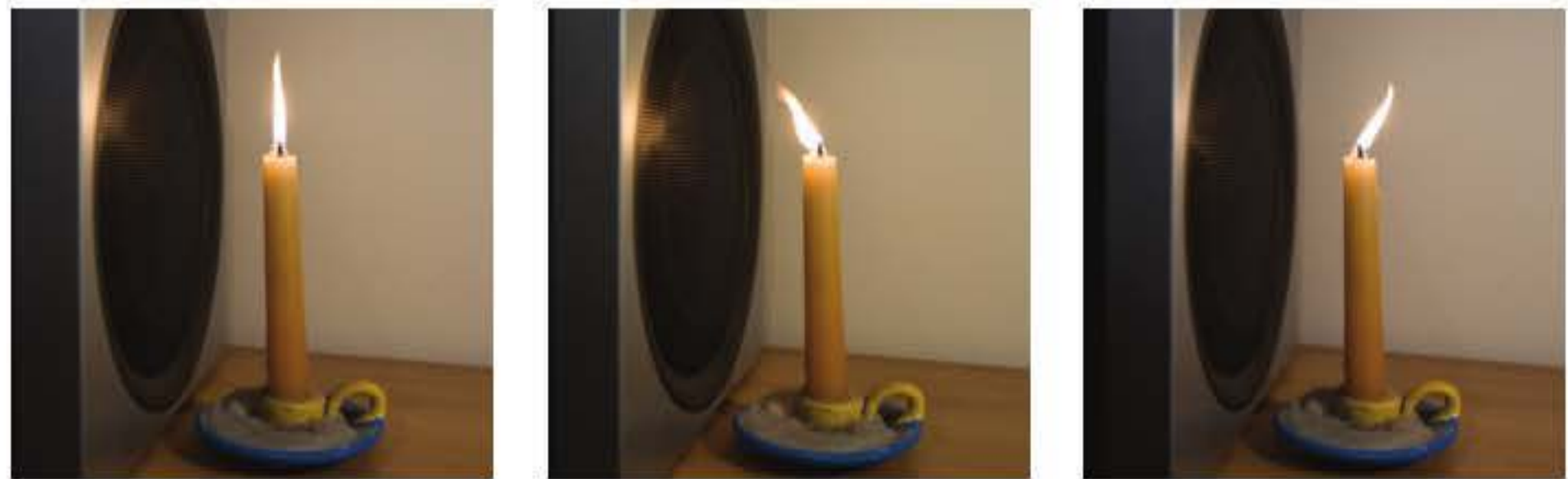
FIGURE 2.1.6 The motion of a flame in front of a loudspeaker is clear evidence of the continuous movement of air backwards and forwards as the loudspeaker creates a sound wave.
