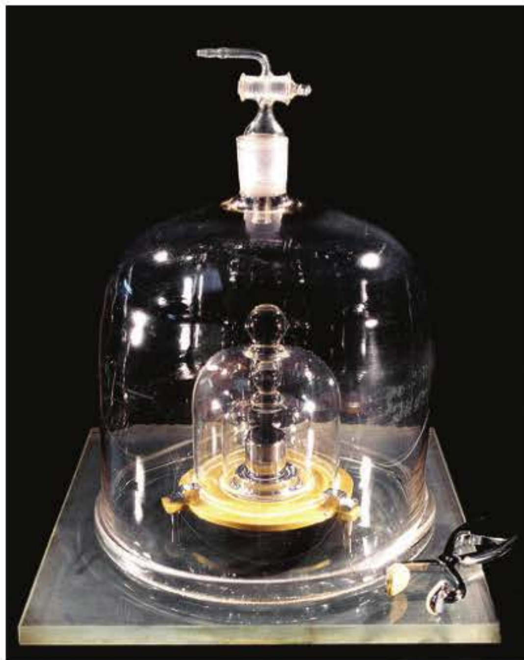
FIGURE 11.5.1 Up until 20 May 2019 all mass in the world was compared to this small piece of platinum–iridium alloy held in a sealed vault in Paris.
