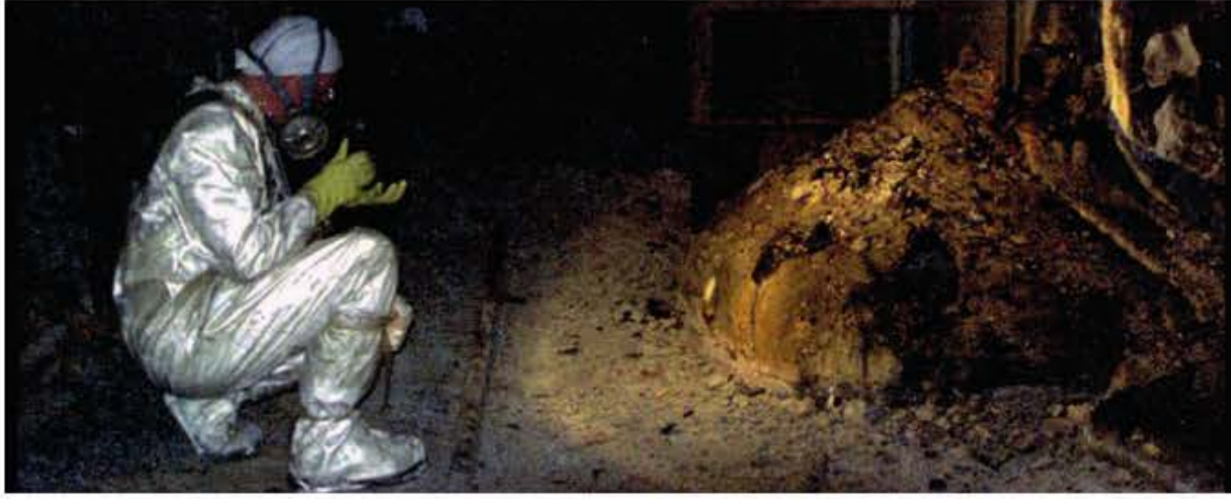
FIGURE 7.2.13 The structure known as the 'Elephant's Foot' at Chernobyl is a solidified radioactive 'lava' of nuclear fuel, melted concrete and other materials.
