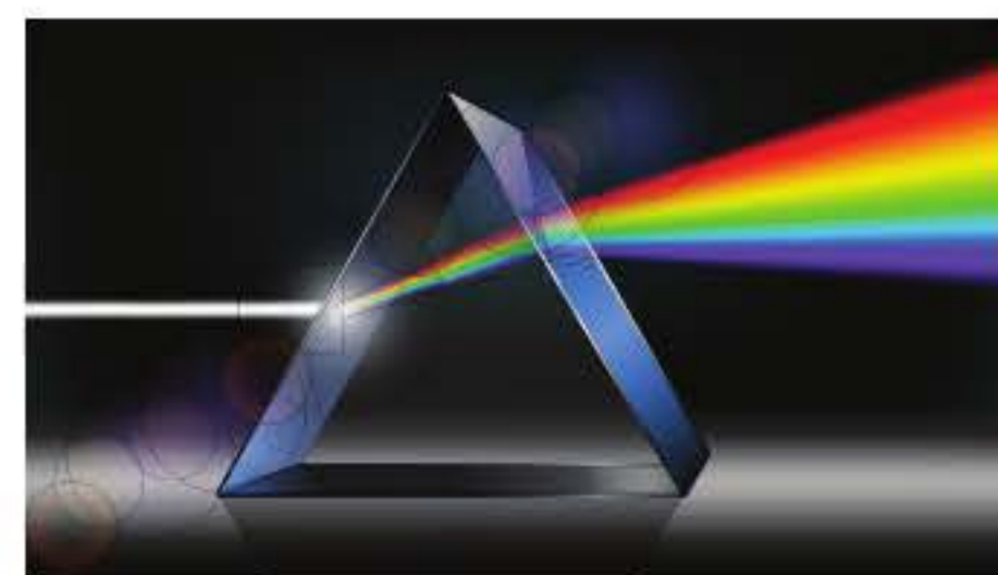
FIGURE 3.2.1 When white light enters a prism, it is split into its component wavelengths or colours.
