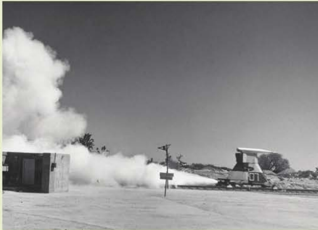
FIGURE 11.2.3 The rocket-powered sled used to test the effects of acceleration on humans
