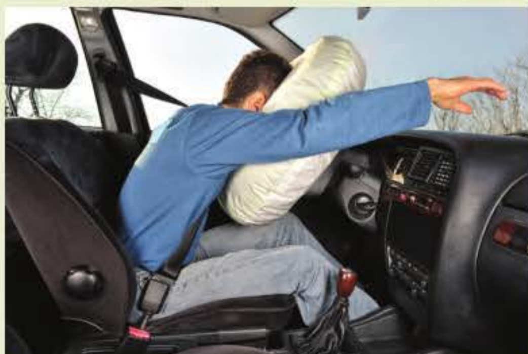
FIGURE 12.6.3 Airbags can prevent injuries by extending the period of time it takes the car's occupants to stop.
