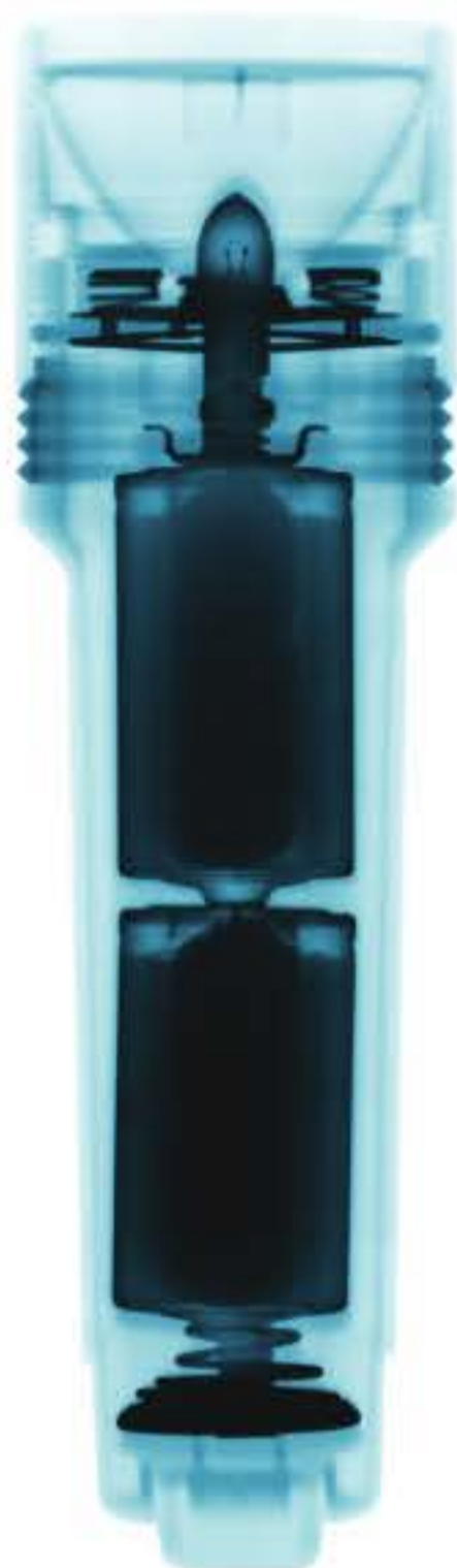
FIGURE 8.3.2 An X-ray image of the internal structure of a torch. The bulb and two batteries are clearly visible.
