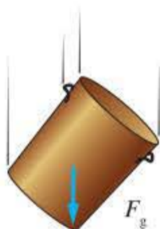
FIGURE 12.3.5 When the bin is in mid-air, there is an unbalanced force due to gravity acting on it so it accelerates towards the ground.
