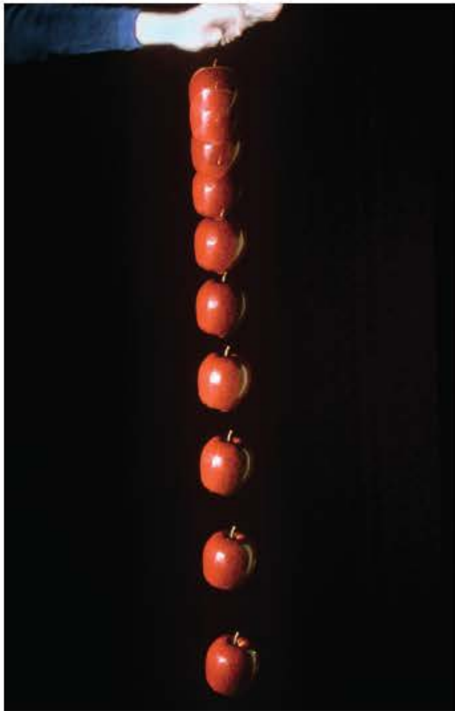
FIGURE 11.5.5 A stroboscopic image of an apple in free fall. The time elapsed between each image of the apple is the same but the distance it travels increases, which shows the apple is accelerating. Without air resistance, this rate of acceleration is the same for all objects.
