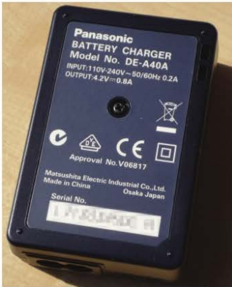
FIGURE 9.3.7 The double square symbol indicates that this appliance has double insulation and does not use an earth connection.
