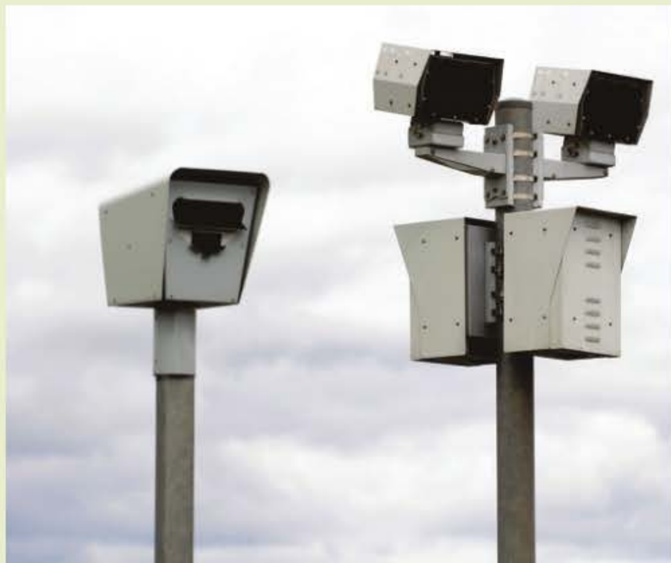
FIGURE 11.1.6 Speed cameras on poles
