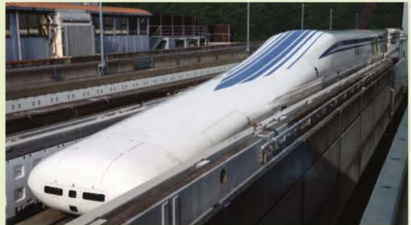
FIGURE 9.1.12 Maglev train. This part of Japan's rail system uses superconductors to provide the magnetic levitation of the train and carriages.
