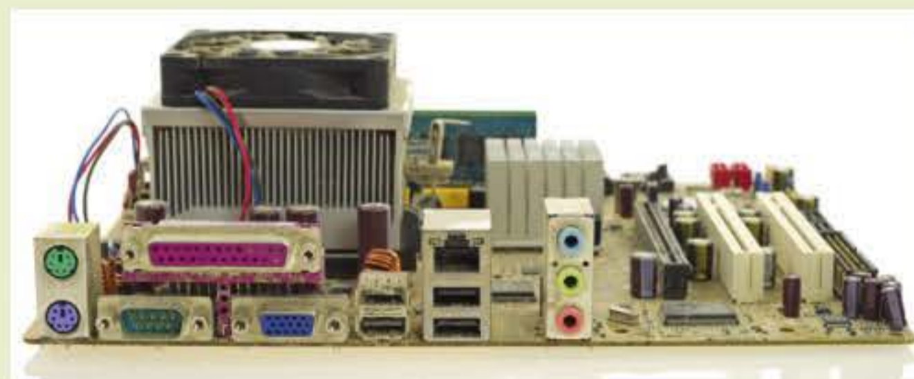
FIGURE 8.4.1 The fan in this computer motherboard circulates air around the electrical components to cool them down.
