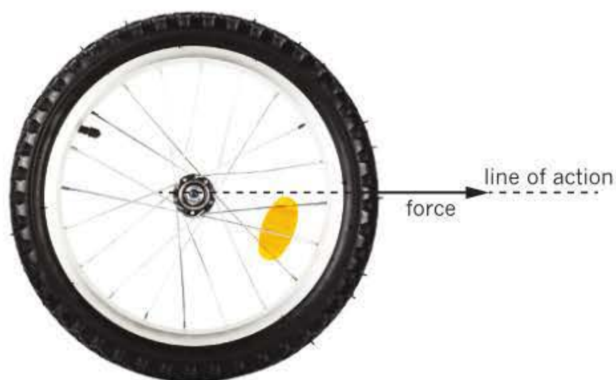
FIGURE 14.1.4 When the line of action of the force passes through the pivot point, the wheel will not turn.
