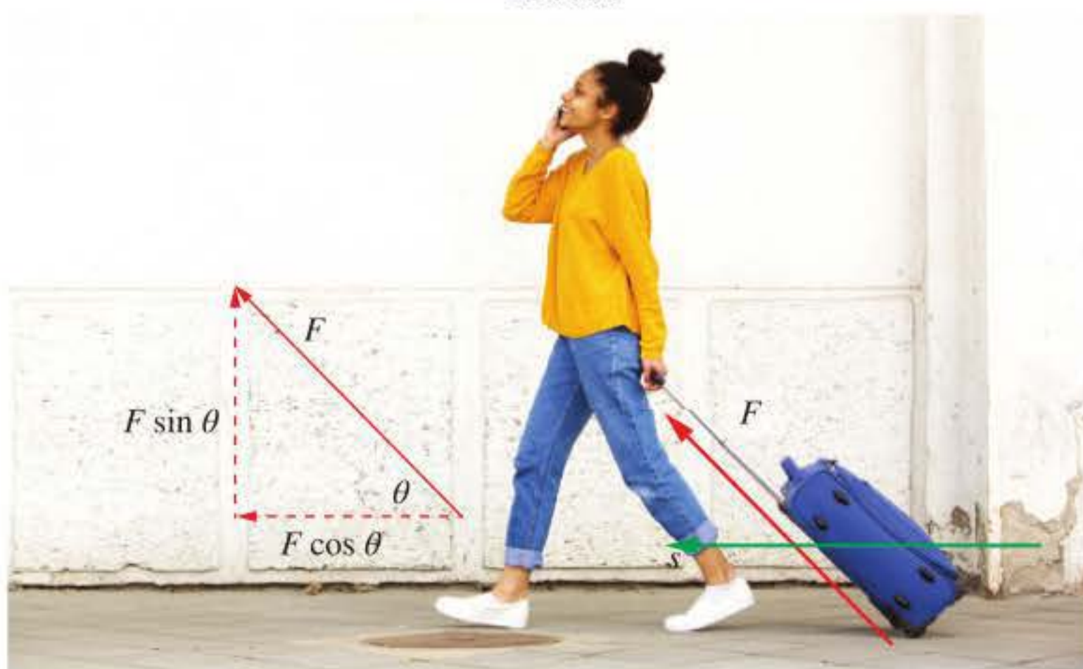
FIGURE 13.1.5 The force applied by the person pulling the suitcase can be resolved into a horizontal force and a vertical force.
