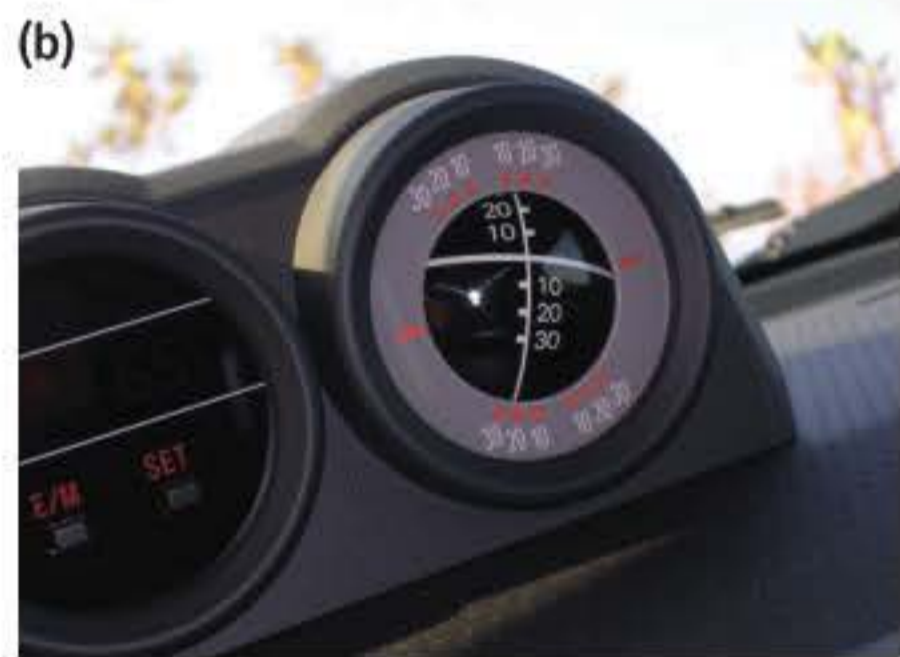
FIGURE 14.3.8 (a) The car on the incline is in stable equilibrium, while the heavily laden truck on the same incline could topple. The force due to gravity vector is outside the lower point of support for the truck, so there is no reaction force from the road to the higher wheel. (b) Modern four-wheel drive cars and tractors have inclinometers to warn the driver if the vehicle is in danger of tipping.
