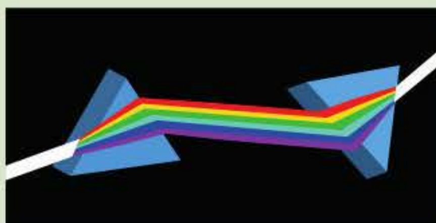
Newton's double prism experiment showed that white light is made up of its component colours.
