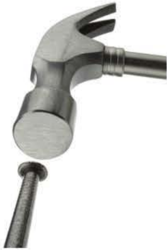
FIGURE 12.3.1 A hammer hitting a nail is a good example of an action–reaction pair and Newton's third law.
