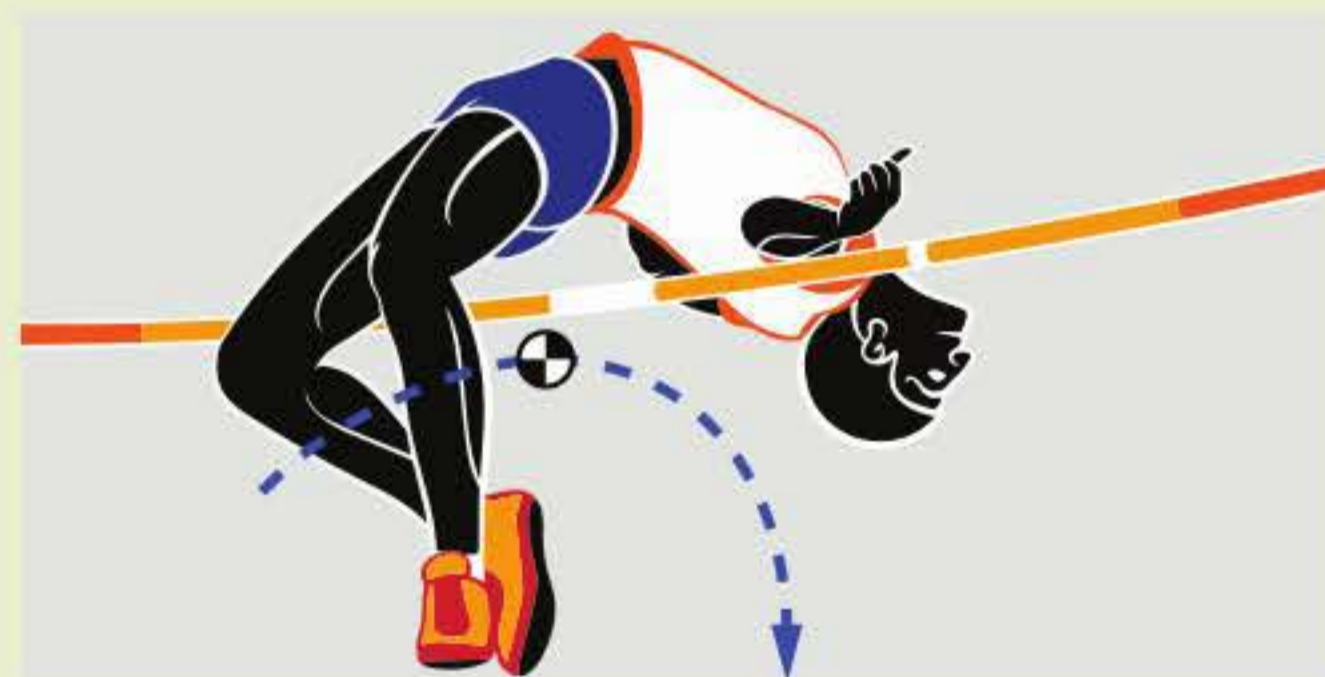
FIGURE 13.2.6 The path of the centre of mass of the high jumper (shown by the dashed curve) passes below the high jump bar.
