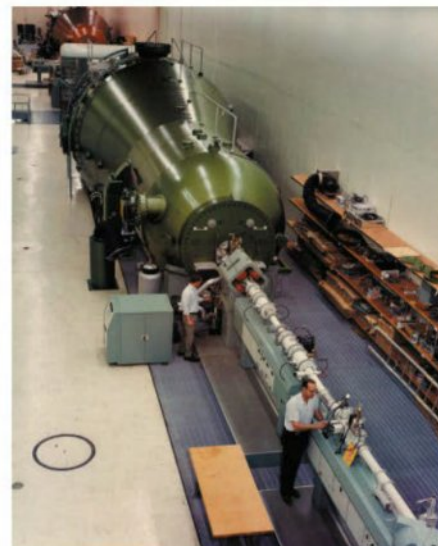
FIGURE 6.3.2 This tandem Van de Graaff accelerator uses two generators to produce beams of charged particles that are accelerated by potential differences of up to 10 million volts.
