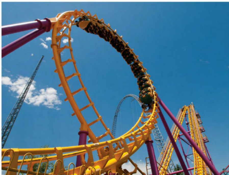
FIGURE 2.4.6 The thrill seekers on this rollercoaster ride don't fall out when upside down because the centripetal acceleration of their cart is greater than 9.8\text{ m s}^{-2} down.
