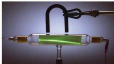
FIGURE 6.3.5 Electron beam being deflected by a magnet
