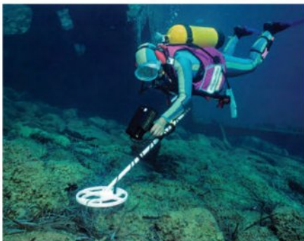
FIGURE 7.2.2 A diver using a metal detector, first invented by Heinrich Lenz. If the coil of the detector passes over a metal object, an EMF is induced. This creates a detectable change in current.
