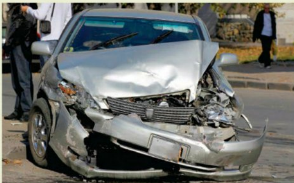
FIGURE 3.2.6 Cars are designed with weak points in their chassis that enable them to crumple in the event of a collision. This extends the time over which they come to rest and so reduces the size of the forces acting on the occupants.
