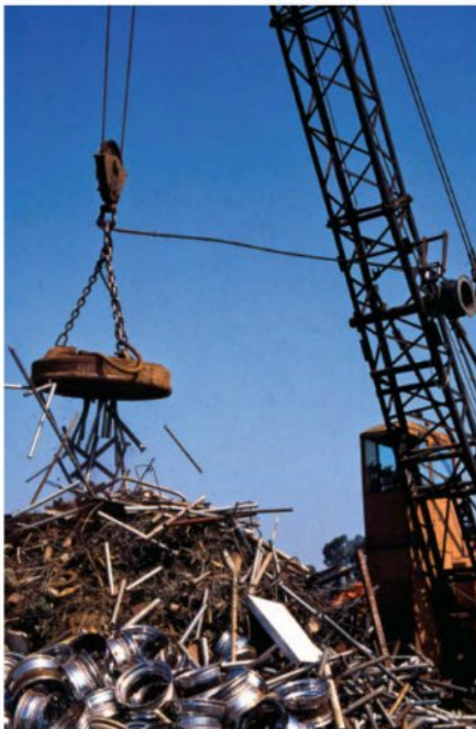
FIGURE 5.3.18 A large electromagnet is being used to lift waste iron and steel at a scrapyard. Valuable metals such as these are separated and then recycled.
