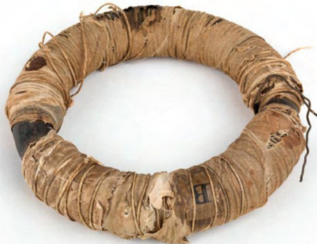
FIGURE 7.1.1 Michael Faraday's original induction ring. It had two coils of wire—insulated from one another—wound around an iron ring. Passing a current through one coil and turning the current off induced a short-lived voltage in the second coil. The ring is on display in the Faraday Museum at the Royal Institution in London.
