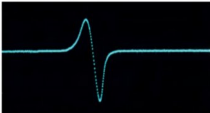
FIGURE 7.2.1 An oscilloscope trace showing the EMF induced as a magnet is dropped through a coil. Notice the spike as the magnet enters the coil and the other spike as the magnet passes out of the coil.
