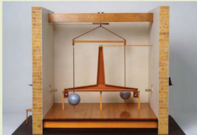
FIGURE 4.1.3 A model of the torsion balance that Henry Cavendish used to measure the small twisting force created by the gravitational attraction of lead balls.
