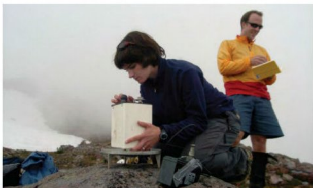
FIGURE 4.2.6 A gravimeter can be used to measure the strength of the local gravitational field.
