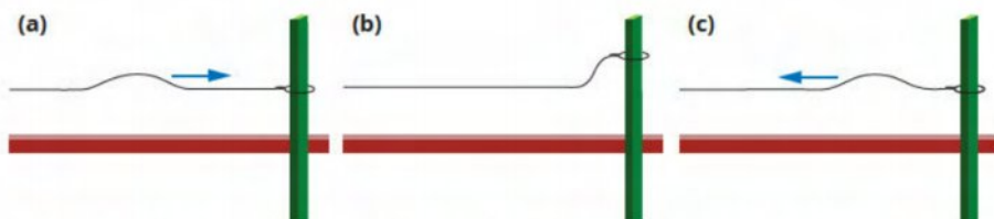
FIGURE 8.2.3 (a) A wave pulse moves along a string to the right and approaches a free end of the string at the post. (b) On reaching the post the free end of the string is free to slide up the post. (c) No inversion happens and the wave pulse is reflected back to the left on the same side of the string, i.e. there is no phase reversal on reflection from a free end.
