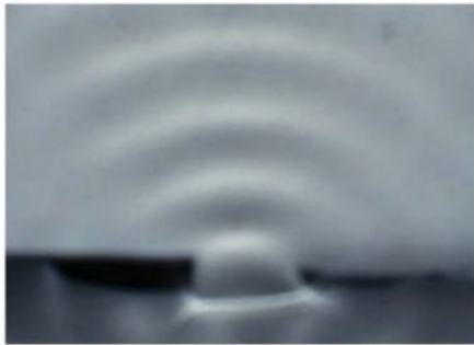
FIGURE 8.3.4 Water waves will diffract (bend) as they pass through narrow openings. Sound waves diffract as well, allowing you to hear around corners.
