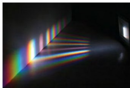
FIGURE 8.3.8 A diffraction grating disperses white light into its component colours.
