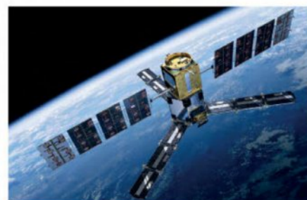
FIGURE 6.1.14 A low-orbit satellite called the Soil Moisture and Ocean Salinity (SMOS) probe was launched in August 2014. Its role is to measure water movements and salinity levels on the Earth in order to monitor climate change. It was launched from northern Russia by the European Space Agency (ESA).
