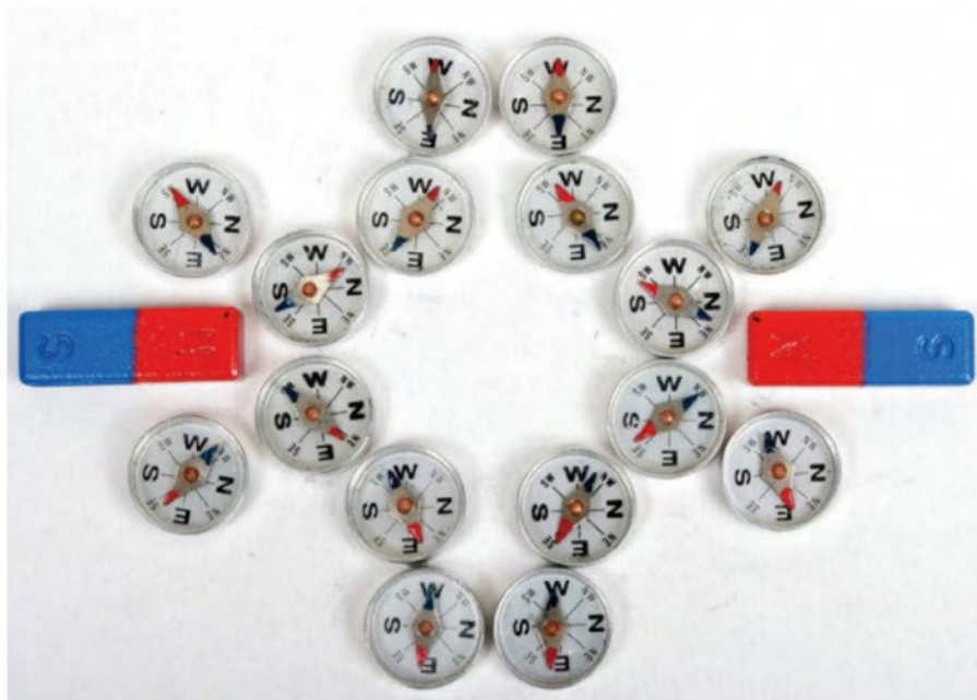
FIGURE 5.3.7 Small plotting compasses are placed around the magnets to help visualise the direction of the field lines.
