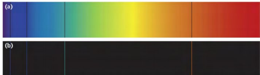
FIGURE 9.3.5 (a) The absorption line spectrum of hydrogen shows a background of the continuous white light spectrum, with black lines that correspond to absorbed wavelengths. The radiation from the Sun has these same black lines, because these frequencies are absorbed by the hydrogen atoms in the outer surface of the Sun. (b) The emission line spectrum of hydrogen shows a black background with lines in the visible spectrum that correspond to the wavelengths emitted by excited hydrogen atoms as they return to the ground state.
