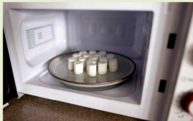
FIGURE 8.3.3 Microwave ovens produce electromagnetic radiation with a frequency of 2.45 GHz, which is the resonant frequency of water molecules.
