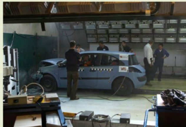
FIGURE 3.2.7 The Australian New Car Assessment Program (ANCAP) assesses the crashworthiness of new cars. This car has just crashed at 50 \text{ km h}^{-1} into a 5 t concrete block. The crumpling effect can be seen.
