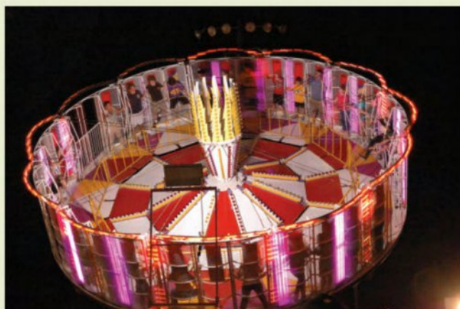
FIGURE 2.2.6 There is a large inwards force from the wall (a normal force) that causes these Gravitron riders to travel in a circular path.
