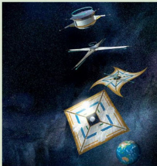
An artist's impression of IKAROS, the first interplanetary spacecraft to use solar-sail technology.
