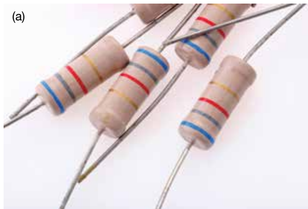
Examples of (a) carbon resistors and (b) a coiled wire resistor
