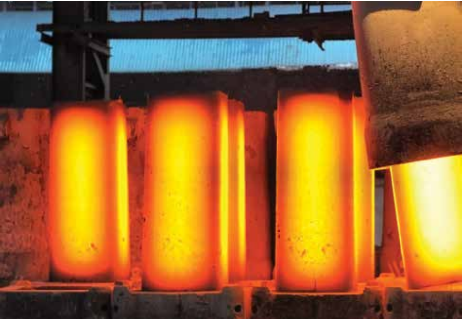
This steel is nearly 1000 °C and has recently been poured in a mould to shape it. The steel will continue to glow until it has cooled to about 400 °C.
