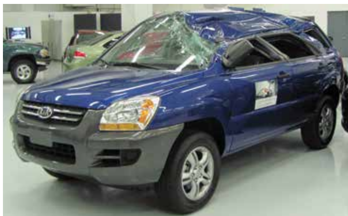
A vehicle that has undergone a roof crush test
