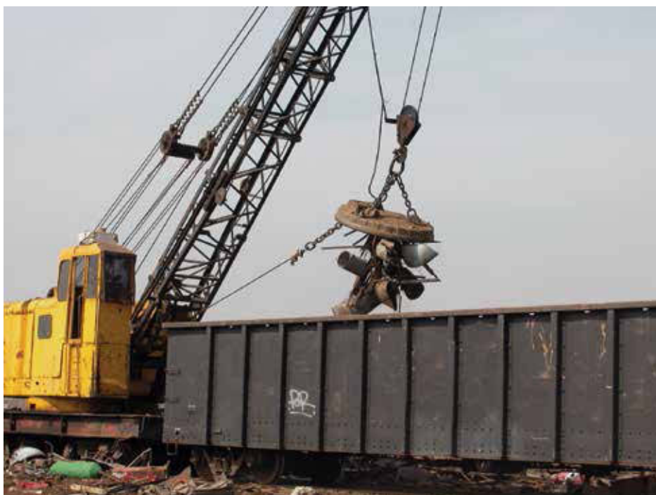
Car parts being lifted by an electromagnet in a car wrecking yard
