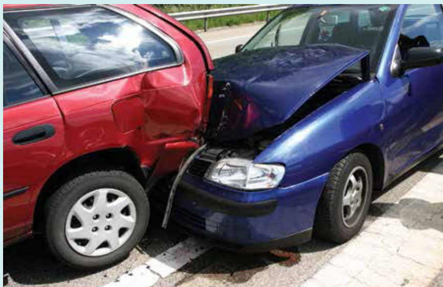
Crumple zones at the front and rear of cars absorb energy and reduce the magnitude of acceleration during an accident.
