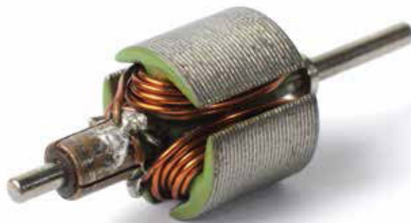
Commutator and coil from a hair dryer
