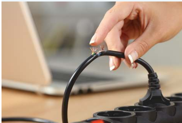
FIGURE 7.13 Frayed electrical cords
