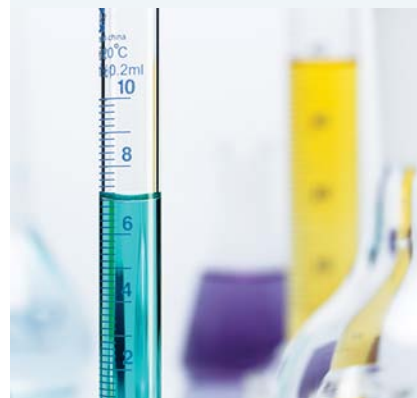
FIGURE 12.48 Liquids should be measured from the bottom of the dip (meniscus) to avoid errors.
