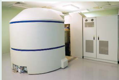
FIGURE 4.16 A cyclotron for radioisotope synthesis in a clinical medical centre
