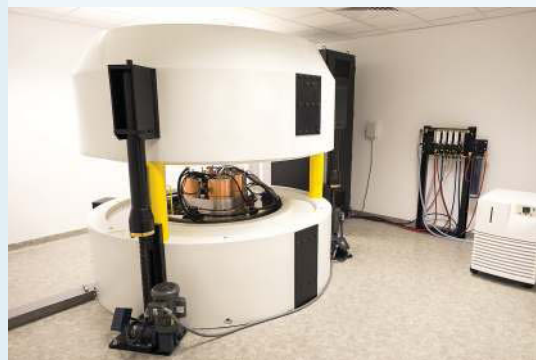
FIGURE 11.6.3 A cyclotron for radionuclide synthesis and isotope production
