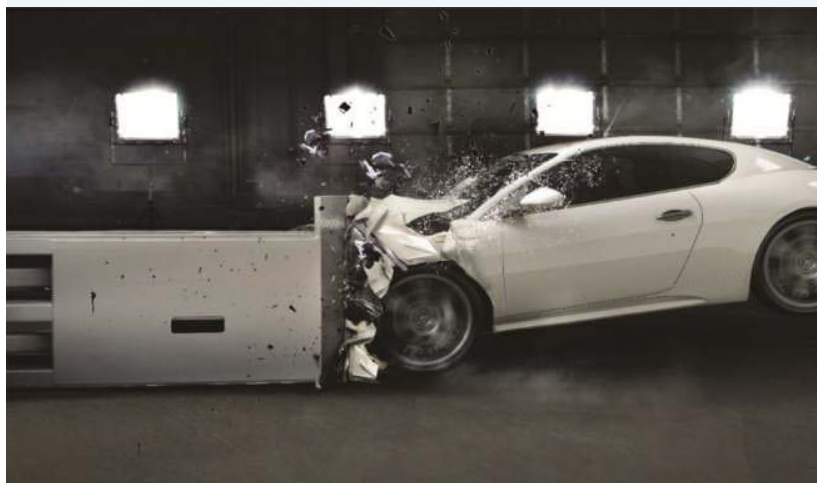
FIGURE 10.1 In this collision the kinetic energy of a car is transferred into many other forms of energy. Energy from the car is transformed into the deformation of the materials that the front of the car is made of, and a large amount of energy is transferred to the object it collides with, the road and the particles of air around the car. Some of the energy is transferred into sound and heat.
