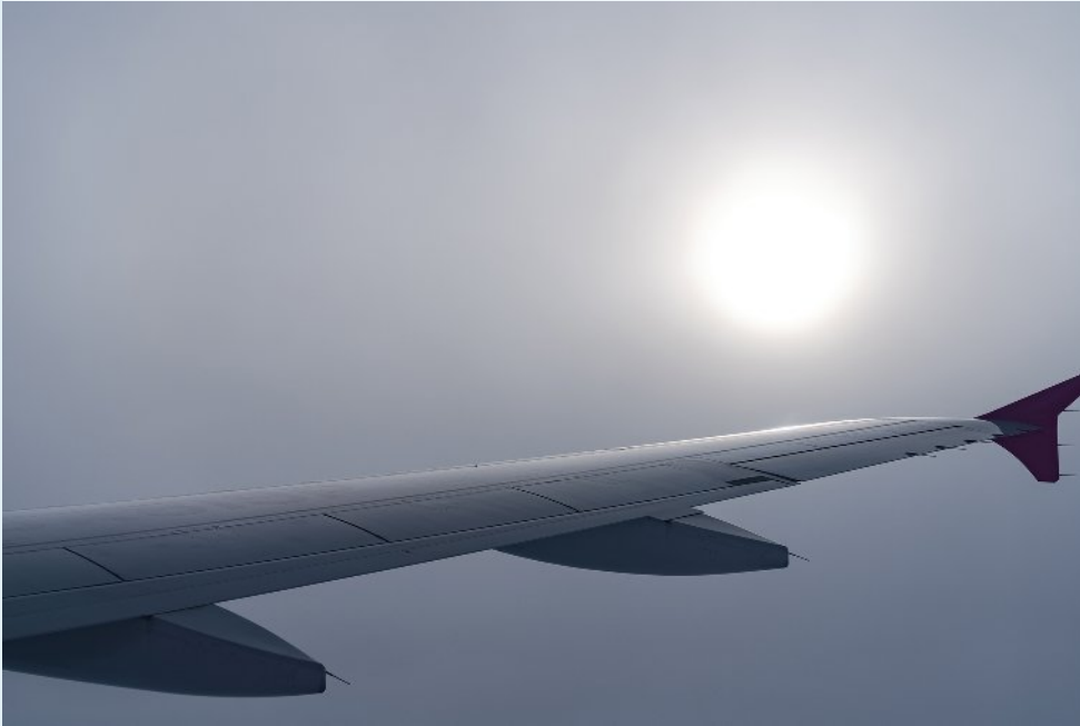
FIGURE 11.3.6 The curved upper surface of an aerofoil forces air to travel more quickly over the top of the aerofoil than below it.
