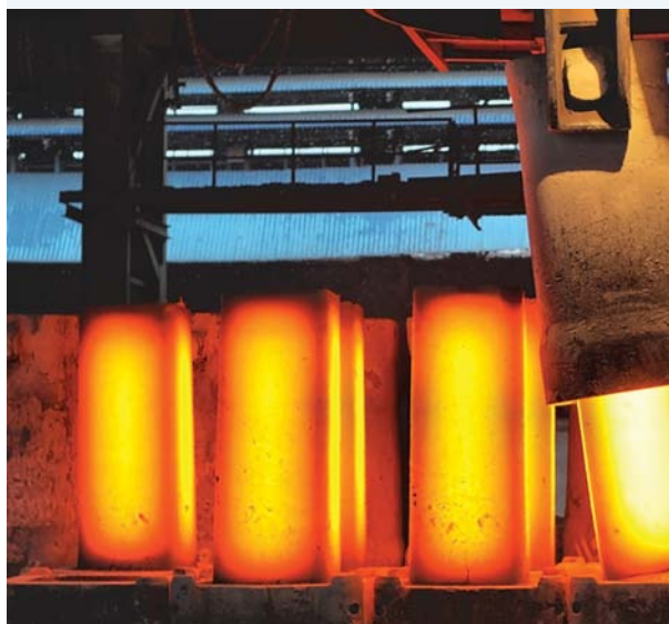
FIGURE 3.8 This steel is nearly 1000 °C and has recently been poured into a mould to shape it. The steel will continue to glow until it has cooled to about 400 °C.
