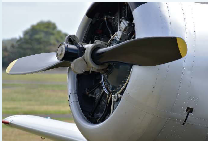
FIGURE 11.3.11 A propeller engine generates thrust by the propeller applying a force to the air, which applies an equal and opposite force back onto the propeller. A propeller-driven aircraft can be thought of as being pulled through the air.
