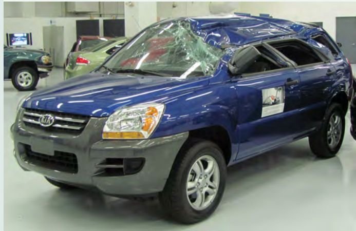
FIGURE 9.28 A vehicle that has undergone a roof crush test
