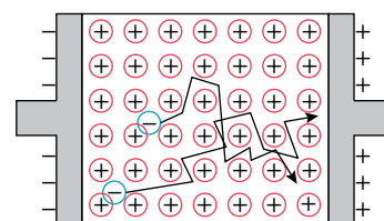
FIGURE 5.7 The electron drift model of current flowing through a metal. Note: Only two of the free electrons have been shown.
