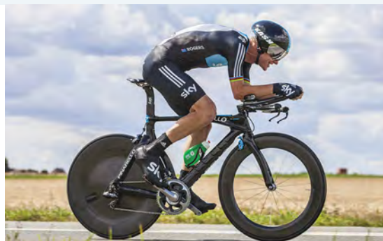
FIGURE 9.6 Racing cyclists reduce the effects of fluid friction (air resistance) by wearing streamlined costumes and using aerodynamically designed bicycles.
