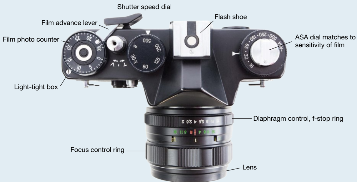
FIGURE 11.9.12 Functional parts of a basic film camera
