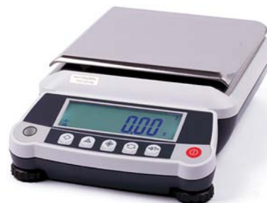
FIGURE 12.51 Top-loading balances measure to a certain number of significant figures.
