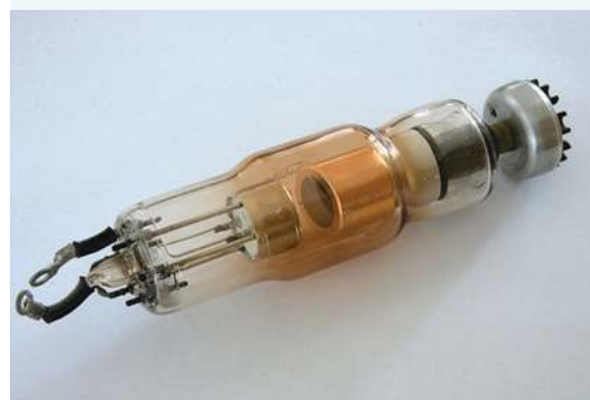
FIGURE 4.1 A dental X-ray tube, with an electron gun on the left-hand side and a tungsten target in the copper sleeve on the right-hand side.
