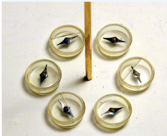
FIGURE 5.21 Magnetic field measurements around a current-carrying wire
