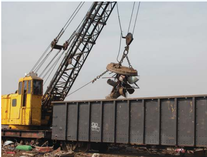
FIGURE 5.18 Car parts being lifted by an electromagnet in a car wrecking yard
