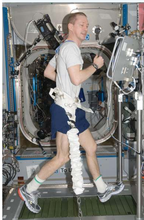
FIGURE 3.11 The cloth-covered stretched springs are pulling the astronaut down so he can exercise on the treadmill.
