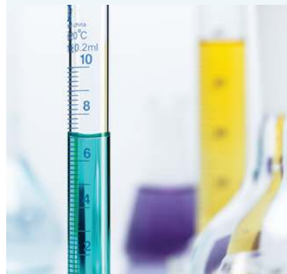
FIGURE 12.37 Liquids should be measured from the bottom of the dip (meniscus) to avoid errors.
