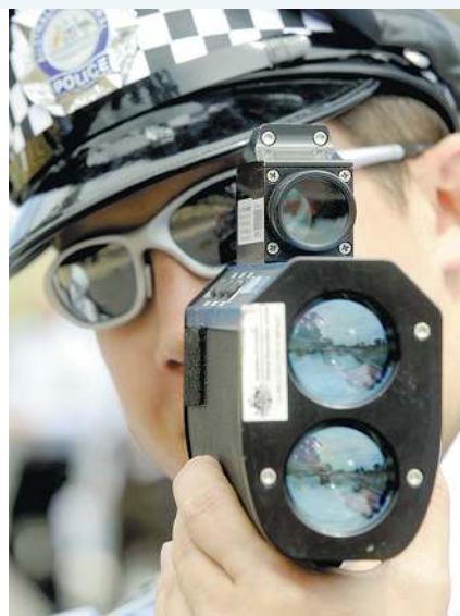
FIGURE 11.5 The radar gun would measure a different speed if it was in a moving vehicle.
