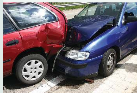
FIGURE 2.14 Crumple zones at the front and rear of cars absorb energy and reduce the magnitude of acceleration during an accident.
