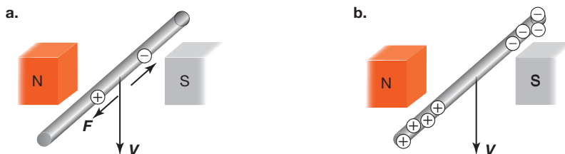
FIGURE 6.3 The magnetic field forces electrons to the far end of the falling rod.
