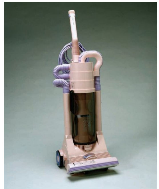
Figure 1.28 Dyson bagless vacuum cleaner, the first vacuum cleaner created by James Dyson. The distinctive Cyclone feature allows continuous suction. Centrifugal force separates dirt and dust from the air, which is then collected in a clear bin. As there is nothing to block the airflow, the system doesn't clog up or lose suction.
