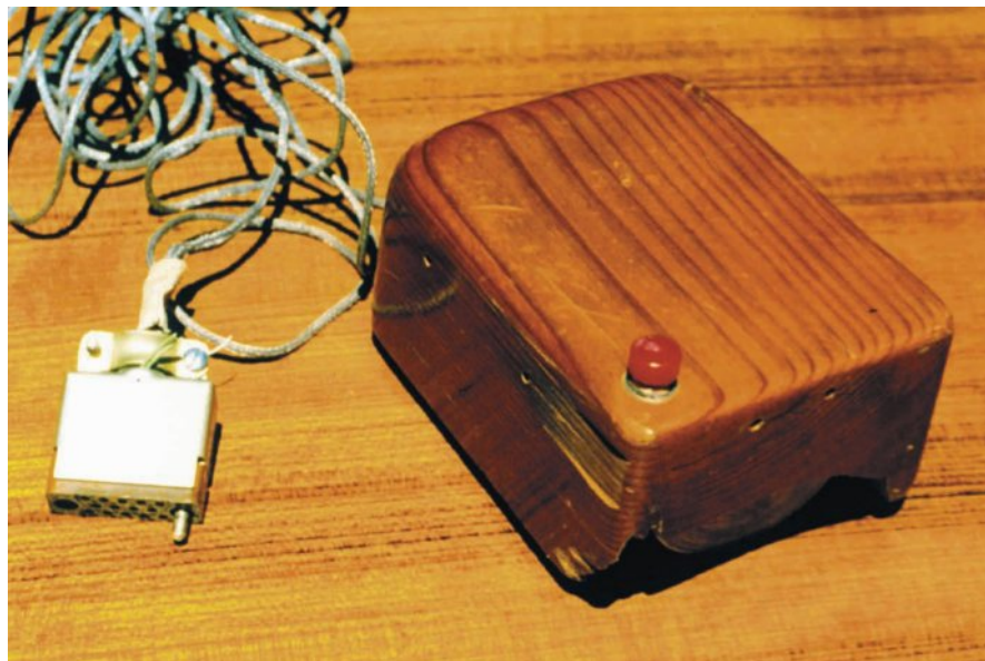
Figure 6.3 Douglas Engelbart's early design of a computer mouse, which was redeveloped by Apple
