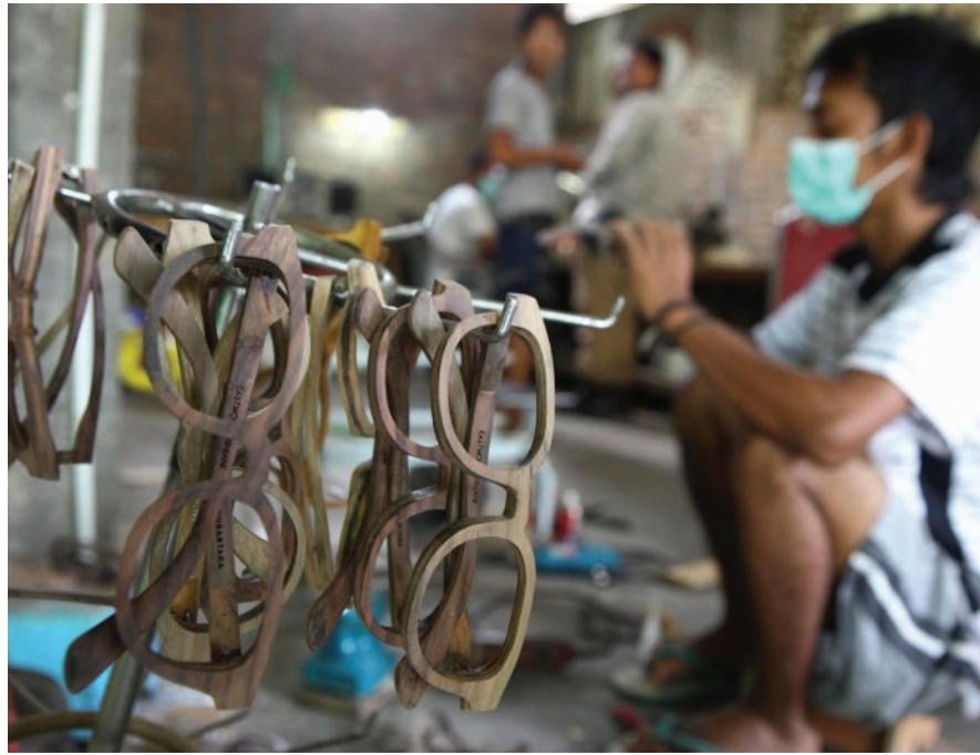
Figure 1.6 A worker making wooden frames for sunglasses using wood that would otherwise go to waste from the furniture industry, mainly teak and rosewood, Indonesia, 2016
