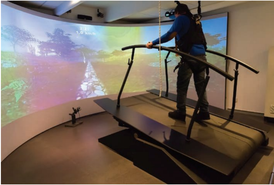
Figure 6A–10 A rehabilitation centre in France is using a new physical therapy system devoted to improving walking through fun exercises with which the patient interacts in real time. It uses a double walkway complete with instruments, a motion capture system, three cameras and EMG, all synchronised with a virtual reality environment.
