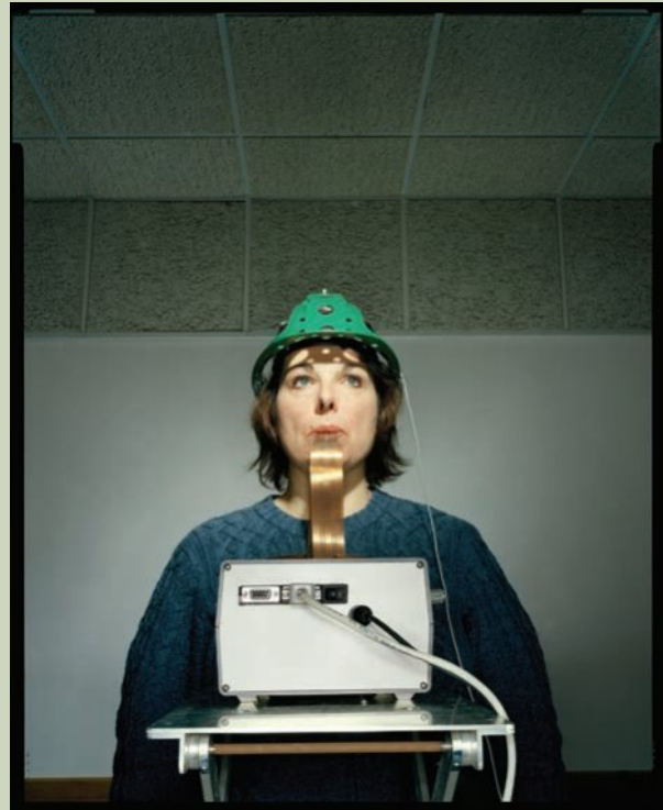
Figure 3C–1 Cheryl using a helmet fitted with motion sensors, connected to a mouthpiece that provides her with feedback sensations on her tongue.
