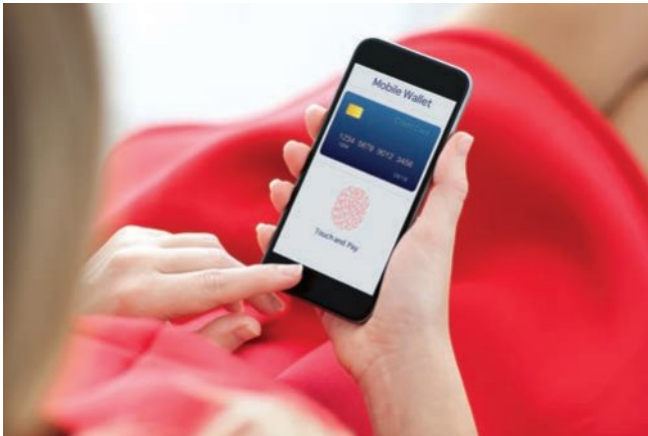
Figure 2A–20 The Touch ID electronic fingerprint recognition on your mobile phone is a valid measure of authentication because it accurately recognises your specific fingerprint before giving you access to the phone.
