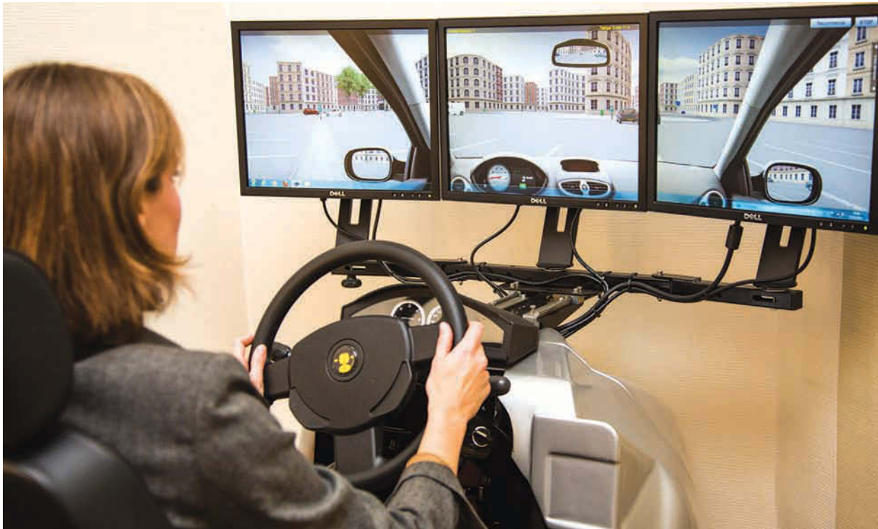
Figure 1.47 A driving simulator used for experimental research. Participant responses to various stimuli may be electronically recorded to collect primary, quantitative, objective data.
