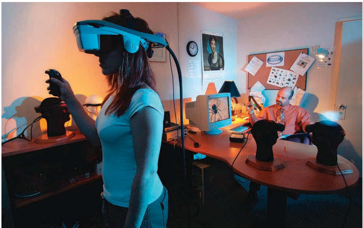
Figure 1.48 Through the development of virtual reality technology, it's now also possible to create almost any type of experience within any type of environment. This virtual reality system is being used to study spider phobia. It contains eye tracking software to study a person's responses when exposed to virtual spiders in a simulated environment.
