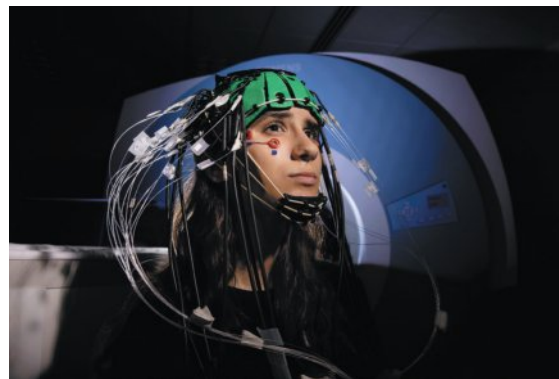
Figure 5.27 A new approach to brain imaging combines functional MRI, electroencephalography and a technique known as EROS, which shines near-infrared light on the scalp to capture brain activity.
