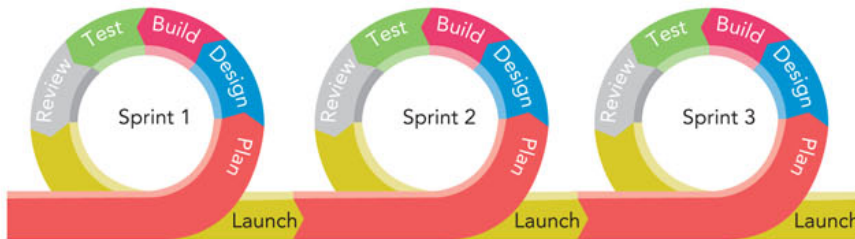
FIGURE 4.28 The Agile software development method is a series of cycles, which continue until the product can be accepted as a minimum viable product (MVP) .
