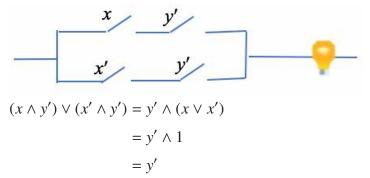
The circuit can be simplified to a y' switch
