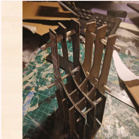
Prototyping combining ideas of the torsion box and the 'chair within a chair'
