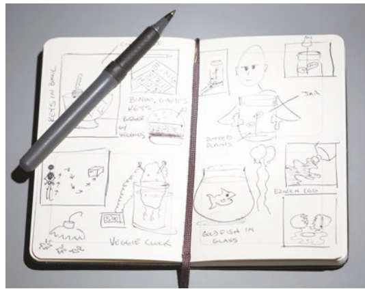
Figure 4.1 Initial industrial design drawings may be quickly generated with pencil or fine liner to allow continuous thought processes.
