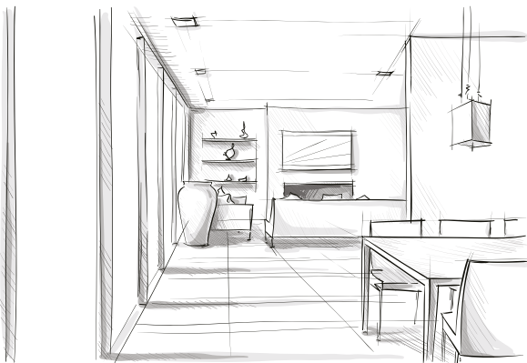
Figure 4.47 One-point perspective drawing of room interior
