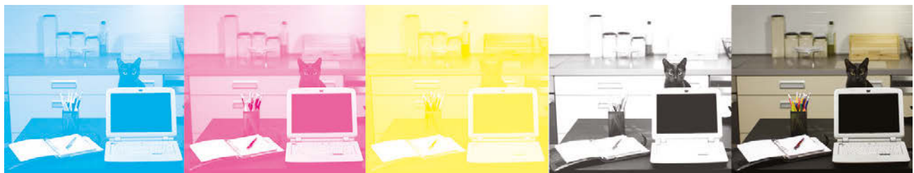
Figure 2.41 CMYK process of overlaying each colour to produce other combinations. When printed on paper, the original image is recreated.
