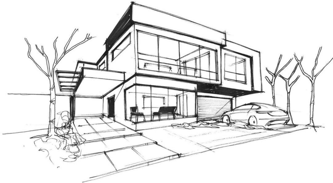
▲ Two-point perspective drawing of an architectural exterior
