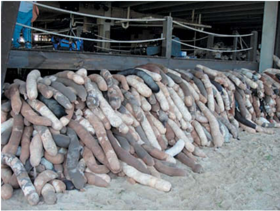
FIGURE 5 Recycled human hair turned into oil-absorbent logs for soaking up oil spills
