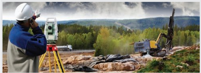
Surveyors use trigonometry to calculate distances and angles between points in three dimensions. Surveyors accurately locate corners for new buildings, boundaries of property for legal ownership, and the placement of roads, bridges, dams, water pipes, power pylons, etc.
