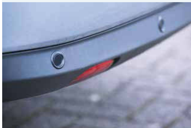
FIGURE 8.12 Sonic motion detectors are used on the bumpers of cars to help the driver detect the distance between the car and another object.
