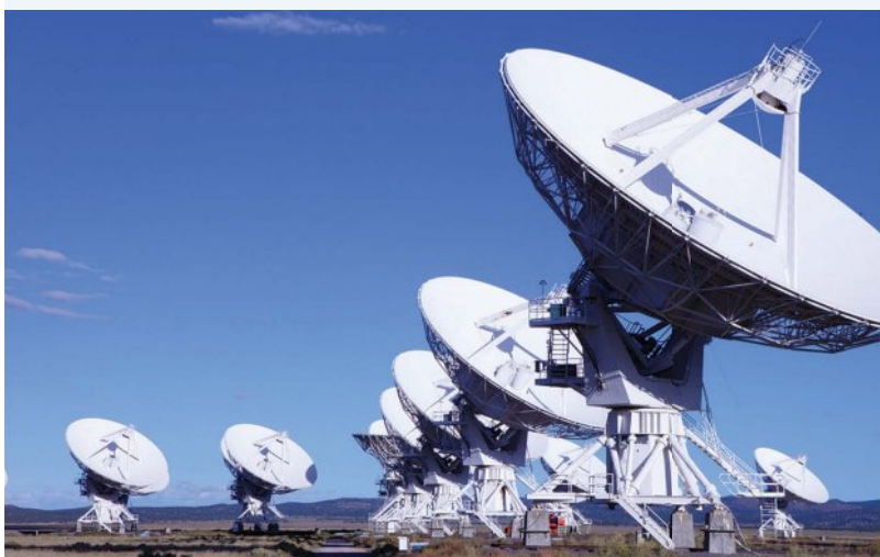
FIGURE 6.20 The Very Large Array in New Mexico consists of 27 dishes, each with a diameter of 25 metres, arranged in a Y shape.
