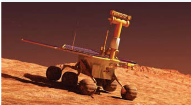
FIGURE 9.55 An example of a Mars rover, which shows the multi-panel solar array spread out like wings
