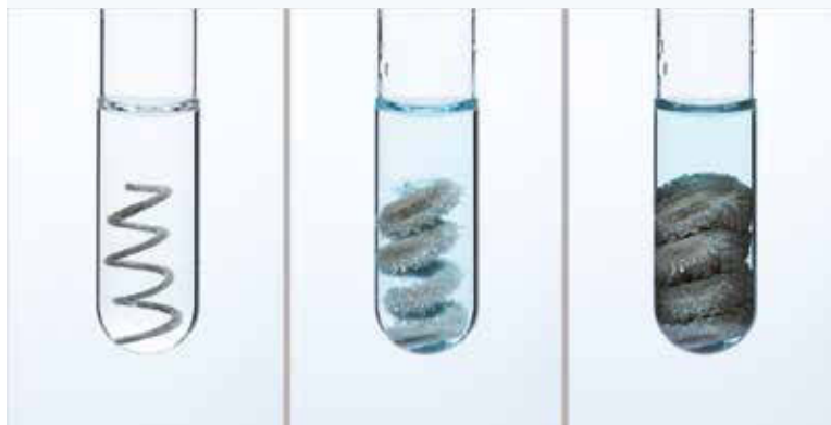
FIGURE 4.36 Production of silver crystals by a displacement reaction between copper atoms and silver ions
