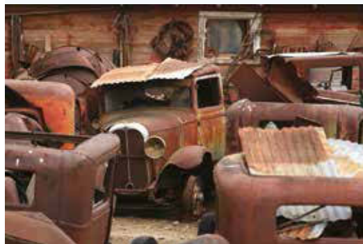
FIGURE 5.16 The rusting of these old car wrecks is an example of corrosion.
