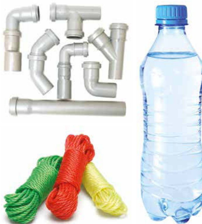
FIGURE 5.30 PVC pipes, polyethylene bottle and nylon rope
