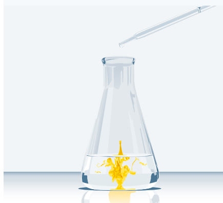
FIGURE 5.9 The formation of the brilliant yellow precipitate, lead iodide, from the colourless solutions of lead nitrate and potassium iodide
