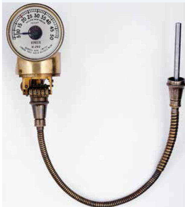
FIGURE 8.13 An older speedometer with a rotating magnet to help detect speed
