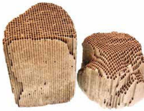
FIGURE 5.39 The honeycombed surface of catalytic converters helps to maximise their surface area and help convert harmful gases into harmless ones.
