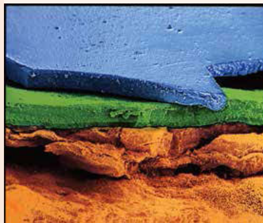
FIGURE 11.43 An electron scanning micrograph of a flake of rusty paintwork; no metal is visible. The blue top layer is a layer of respray paint. It is badly bonded to the original paint, which has three layers of green and orange. The bottom orange crystalline region is rust. This evidence may help to convict a criminal of re-birthing a car.
