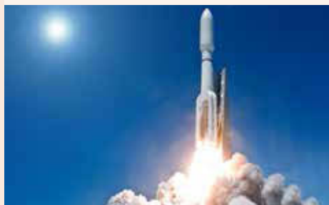
FIGURE 8.25 The rocket pushes away the exhaust gases, and the exhaust gases push the rocket forwards.
