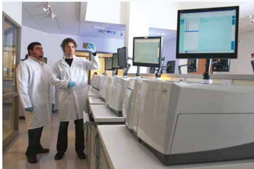
FIGURE 2.50 A DNA sequencing machine. These machines are capable of processing huge numbers of DNA sequences. One machine can sequence 400 to 600 million bases over a 10-hour run.
