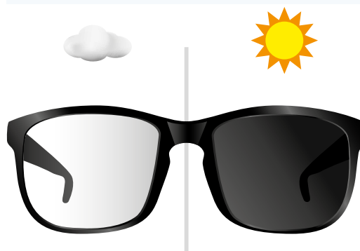
FIGURE 5.18 Photochromic lenses darken in bright sunshine and lighten in areas of low light.
