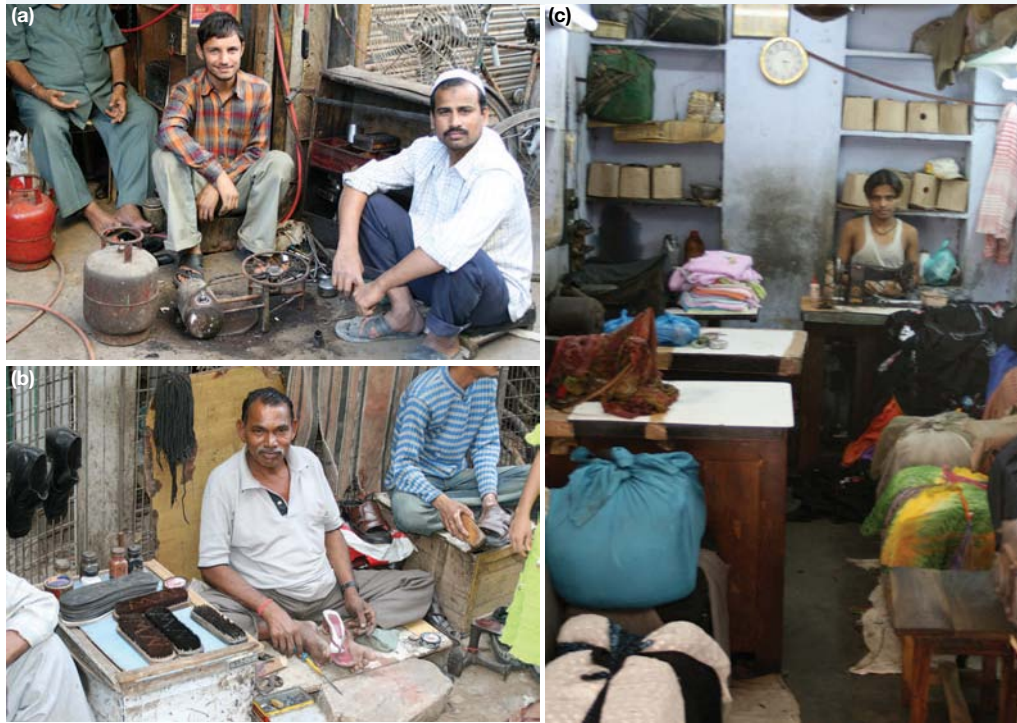
FIGURE 6 As with many other small shops in Old Delhi, the welder (a) works with old homemade equipment. (b) The cobbler repairs shoes with a minimum of equipment, using his feet as a vice. (c) The tailor uses an old sewing machine, operated by a foot pedal.
