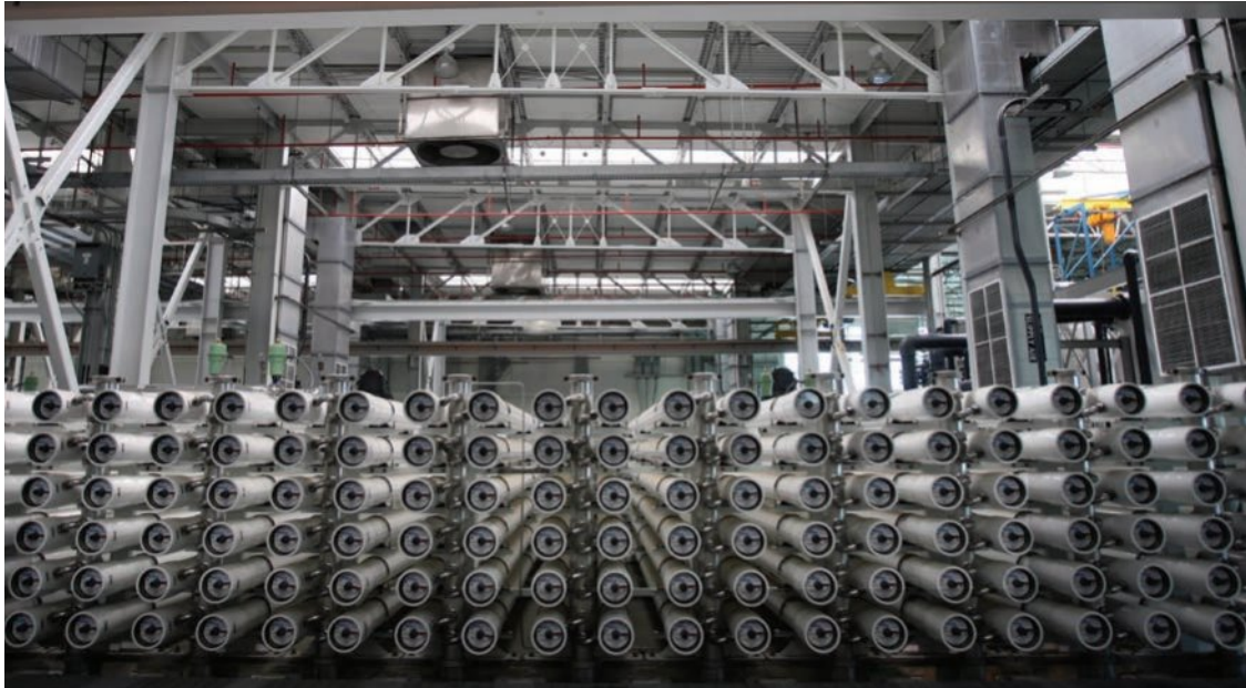
▲ Figure 7.22 This photograph shows the pressure vessels that are used to purify wastewater in Orange County, California
