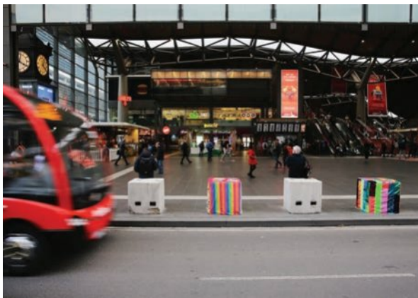
▲ Figure 10.48 Southern Cross Station has concrete bollards so that cars cannot drive into the station from the road
