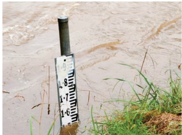
▲ Source 2.9 A common measurement of water levels seen today, based on the design principles of the Nilometer
