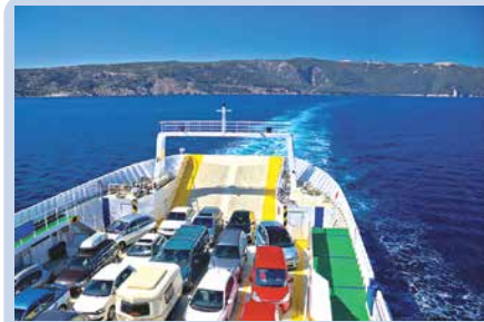
A small car has a mass of about 1 tonne. A vehicle ferry operator must keep the ship stable by balancing the mass of vehicles as the ferry is loaded and unloaded.
