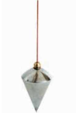
A plumb bob shows the direction of vertical
