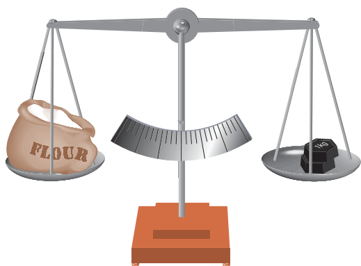
FIGURE 8.9 The two-kilogram bag of flour will always balance the two standard kilogram weights.
