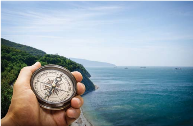
FIGURE 8.31 A compass contains a small magnet that aligns with the Earth's magnetic field.
