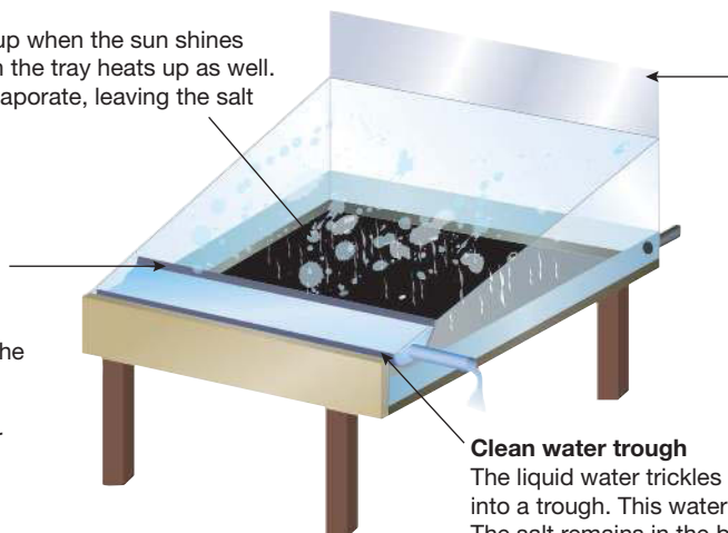
FIGURE 5.19 In solar distillation, the Sun's energy can be used to distill sea water.
