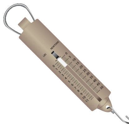
FIGURE 8.10 A spring balance can be used to measure weight.
