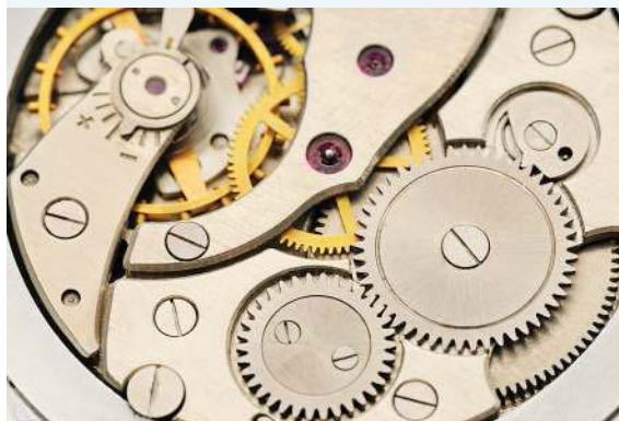
FIGURE 9.25 The gears in this clock form a gear train and allow its three hands to move around its face at different speeds.
