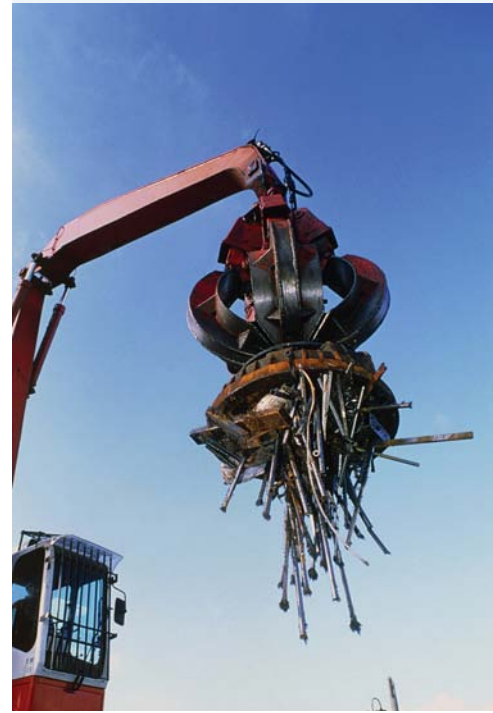
FIGURE 8.33 An electromagnet on a large crane used to lift scrap metal
