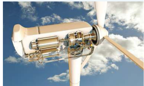
FIGURE 9.23 A combination of gears in a wind turbine allow it to spin quickly.
