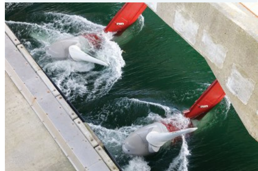
FIGURE 7.17 Turbines harness the tidal currents of the ocean to create electricity.
