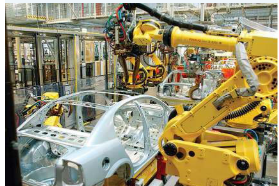
FIGURE 9.34 These robots are used to put the parts of a car body together.
