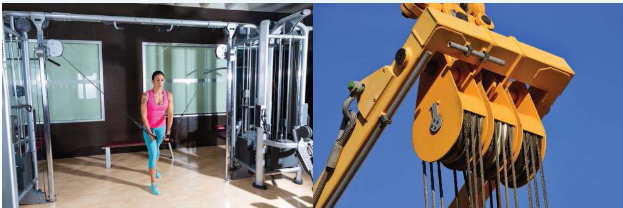
FIGURE 9.20 A pulley changes the direction the effort is needed to lift a load, making it easier.
