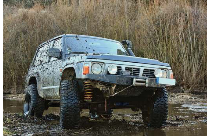
FIGURE 9.33 The front wheel and axle of this vehicle act as a speed multiplier. The outside edge of the wheel turns in a large circle, and much faster than the axle.
