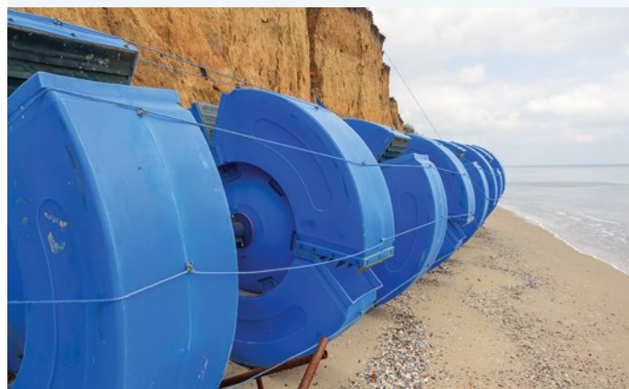
FIGURE 7.16 Part of a wave-powered electricity generator on the shore. Notice the fins inside the turbines that are caught by the waves.
