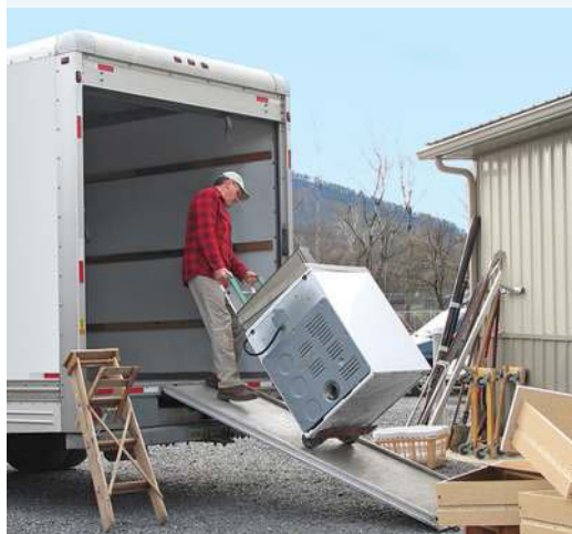
FIGURE 9.11 Lifting a heavy object is made much easier with a ramp.
