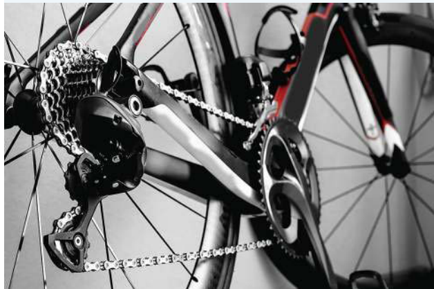
FIGURE 9.24 On a bicycle, the driving gear is moved by pedalling. This causes the driven gears to move.
