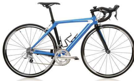
FIGURE 9.30 Gears on a bicycle usually act as speed multipliers.
