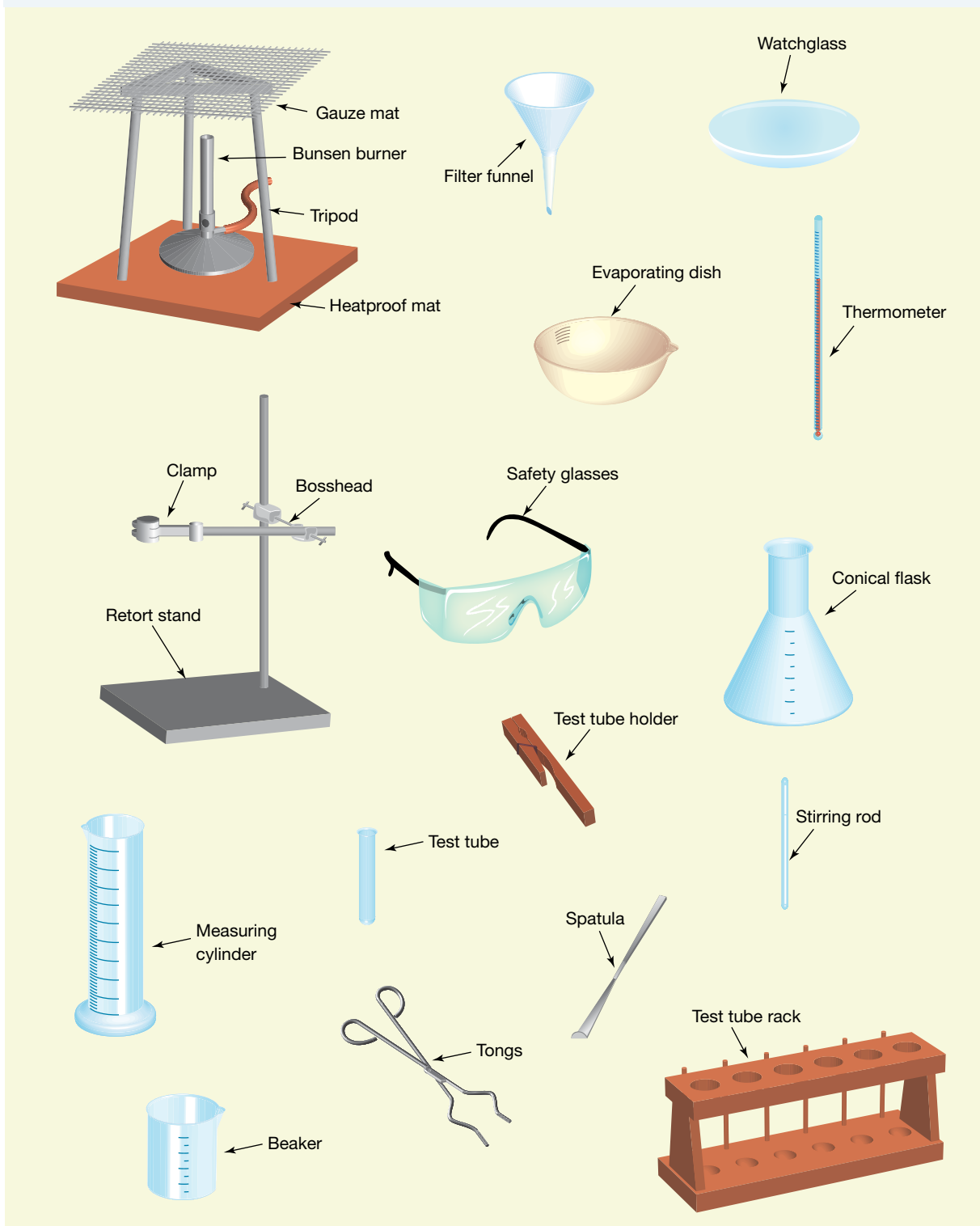
FIGURE 1.9 Some equipment that you are likely to use in the science laboratory
