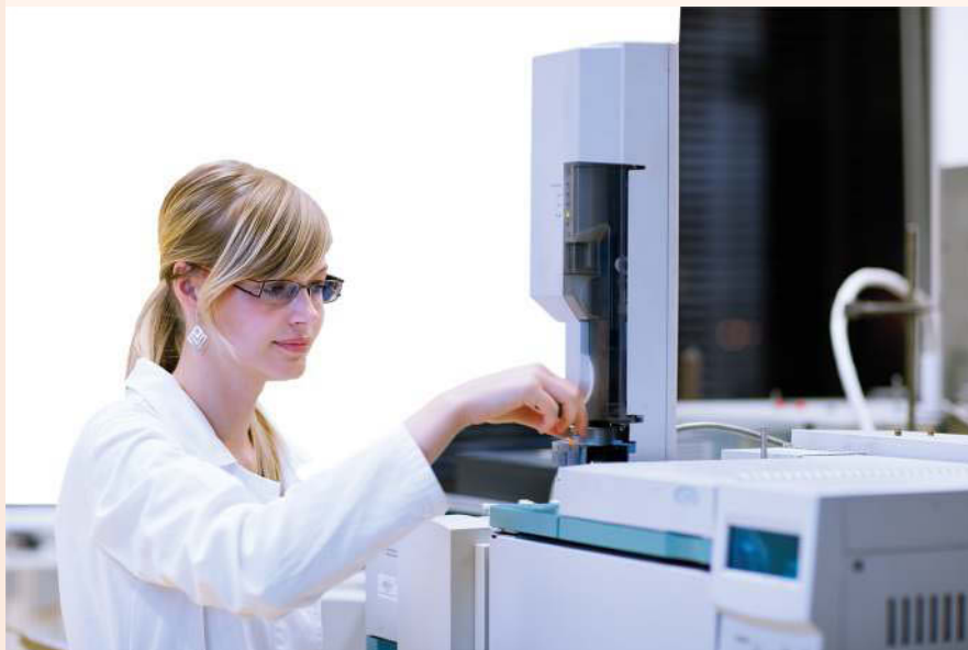
FIGURE 5.21 A chromatograph automatically separates mixtures by chromatography.
