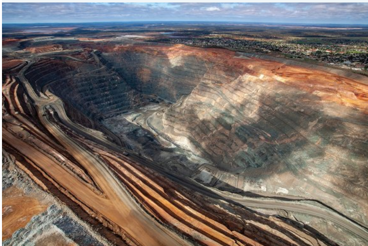
FIGURE 7.4 The Super Pit in Kalgoorlie, Western Australia, is one of Australia's largest open-cut gold mines. In 2020 it was approximately 1.55 km across and 3.7 km long.
