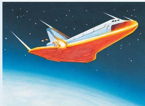
FIGURE 8.20 Damage to Columbia 's ceramic tiles was believed to have caused it to overheat and explode on re-entry in a tragic incident in 2003.
