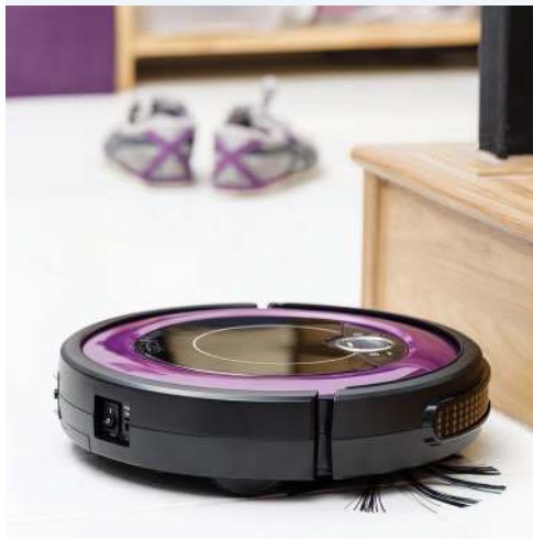
FIGURE 9.35 Most robot vacuums have five motors.
