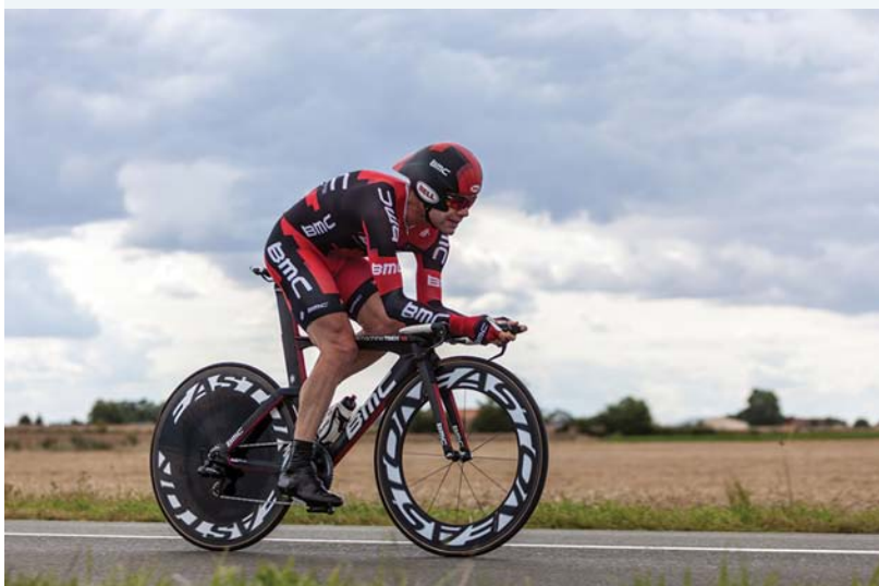
FIGURE 8.18 A racing cyclist's helmet, clothing and bicycle are all designed to reduce fluid friction.
