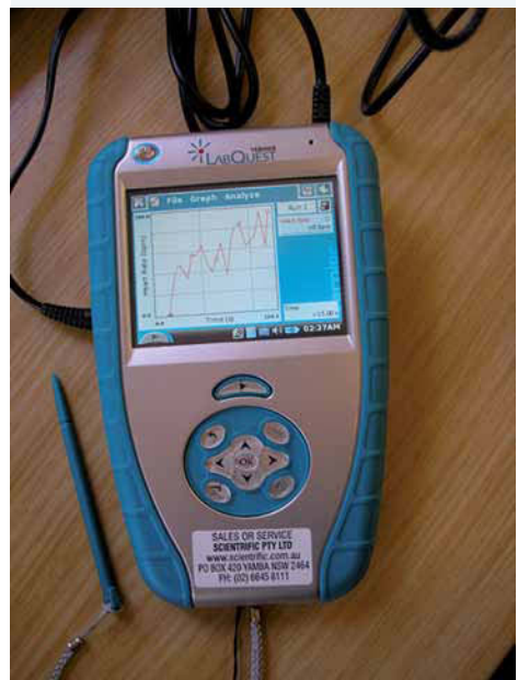
FIGURE 1.24 Some data loggers have their own touch screen and work like mini computers.
