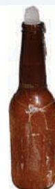
FIGURE 6.24 Oops! The reason why you shouldn't put a bottle full of water in the freezer
