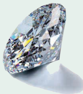
FIGURE 9.7 Faceted diamond, created by grinding a diamond on a spinning lap
