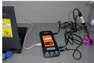
FIGURE 1.25 More basic data loggers require the use of a computer to analyse the results.
