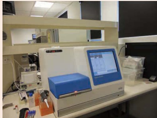
FIGURE 5.90 A time-lapse incubator, which can provide scientists a view of embryos as they develop without disturbing them
