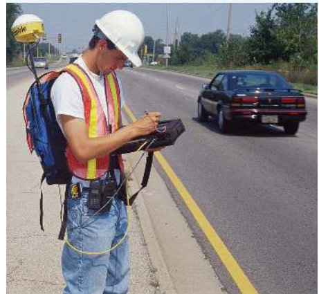
FIGURE 1 Using GPS to survey and record road traffic movements for a local council
