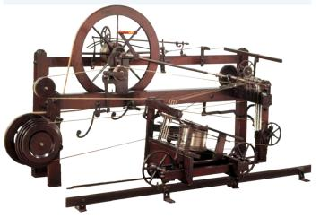
**SOURCE 8** Innovation in the textile industry, 1780s: Textile production began to be centralised in factories. Initially they were built close to rivers to draw on water power, but eventually this became unnecessary as steam power was adopted. Edmund Cartwright developed the power loom, shown in this artwork from c. 1844, which mechanised the weaving process.
