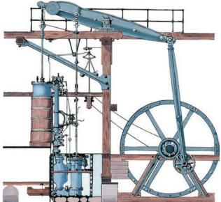
large beam that worked a pump to remove water from underground mines.
