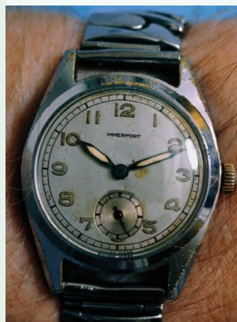
FIGURE 6.12 This watch has been hand painted in luminescent radium paint.
