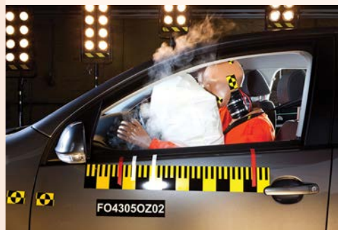
FIGURE 7.9 Airbags inflate as a result of an explosive chemical reaction.
