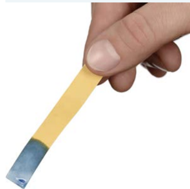
FIGURE 7.13 Litmus paper contains an indicator that turns blue when dipped into a basic solution.
