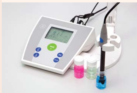
FIGURE 1.24 A pH meter needs to be calibrated regularly to ensure it gives accurate readings.
