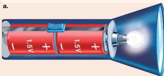
FIGURE 10.13 a. Components of a torch b. Circuit diagram for a torch
