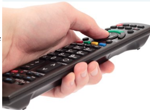
FIGURE 9.39 A gentle push of the button sends infra-red radiation to the television set at 300 million metres per second.
