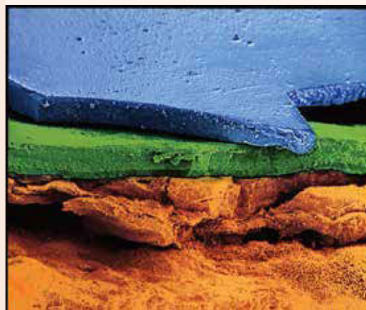
FIGURE 12.43 An electron scanning micrograph of a flake of rusty paintwork; no metal is visible. The blue top layer is a layer of respray paint. It is badly bonded to the original paint, which has three layers of green and orange. The bottom orange crystalline region is rust. This evidence may help to convict a criminal of re-birthing a car.
