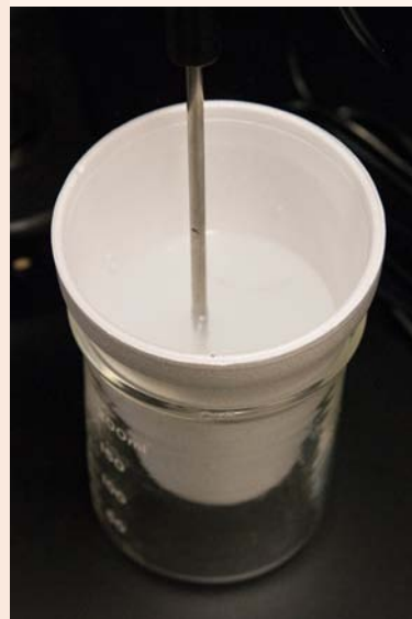
FIGURE 1.30 Place the temperature sensor into the beaker of dilute acid and add the magnesium.
