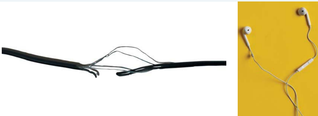
FIGURE 10.4 The cords to earbud headphones carry electricity, not sound. Each cord actually contains two wires. The jack that plugs into the player is composed of four wires, two per earbud.
