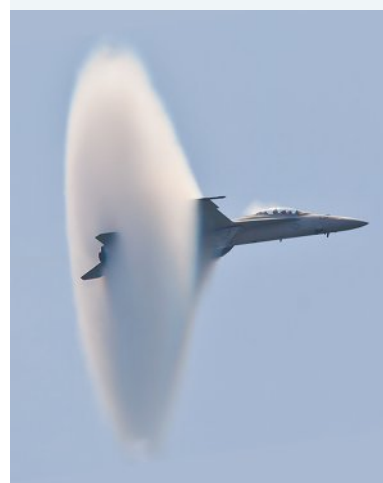
FIGURE 9.24 A jet flying faster than the speed of sound can form a condensation cloud.
