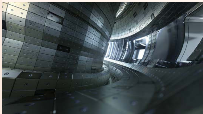
FIGURE 10.58 A tokamak fusion reactor. Powerful magnetic fields hold a superheated gas called a plasma. The magnetic field causes heating in the plasma that can produce collisions between atoms that fuse together to release energy.
