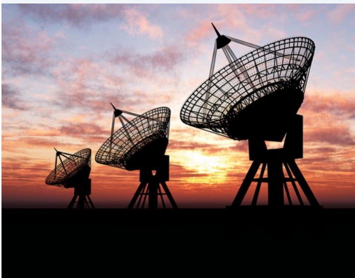
FIGURE 9.71 These antennas receive signals that have been retransmitted by a geostationary satellite.
