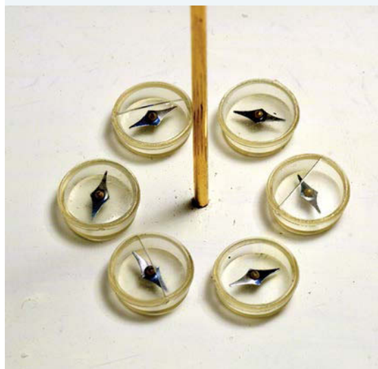
FIGURE 10.40 Without a current the compasses point north, but when the current flows we see evidence of a circular magnetic field.
