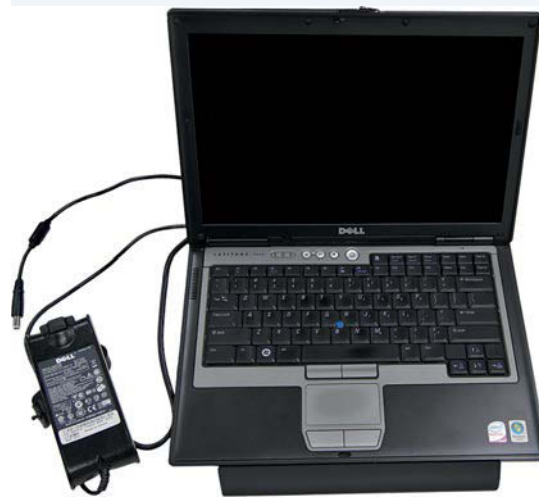
FIGURE 10.55 Some electrical devices require less than the 240 volts supplied by power points. A transformer is used to ‘step down’ the voltage.
