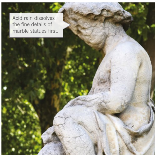
FIGURE 3.2.9 Marble is composed of the base calcium carbonate, which will react with any acid that it comes in contact with. This makes marble statues vulnerable to attack by acid rain.
