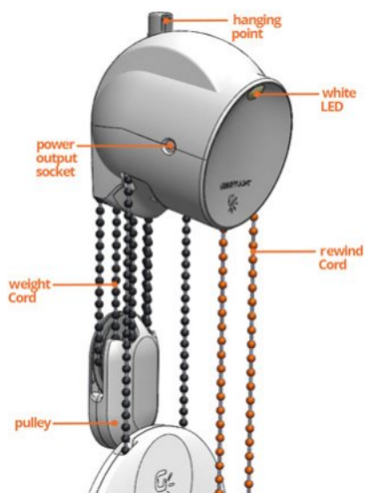
FIGURE 6.4.14 A bag filled with rocks or soil is attached to the bag hook of the GravityLight. The bag falls slowly to the ground and pulls the weight cord through the device. The movement of the cord turns gears, which drive a generator that powers an LED.
