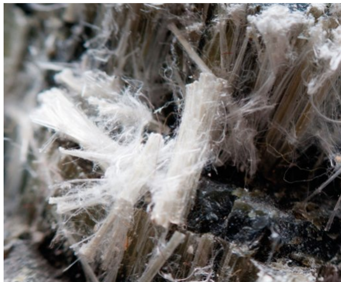
FIGURE 8.3.13 Fibres of asbestos look like cotton wool, but they are not soft. Asbestos fibres are fire-resistant and very strong. They were used to make corrugated roofing, water pipes, fabrics, and brake linings.
