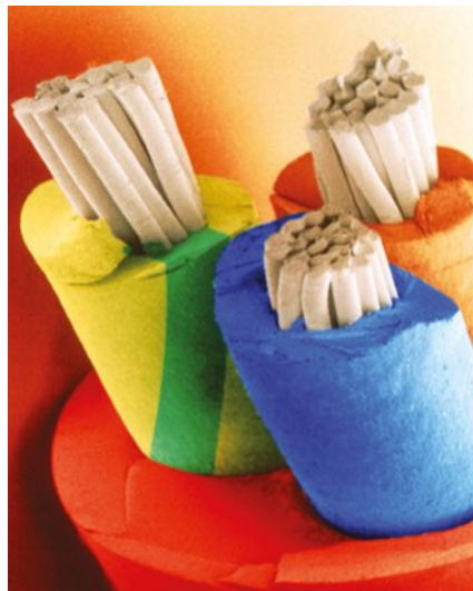
FIGURE 6.2.12 Plastic coating is used to insulate each of the three wires in an electric cable. More plastic coating wraps all the three wires together, insulating them even further.
