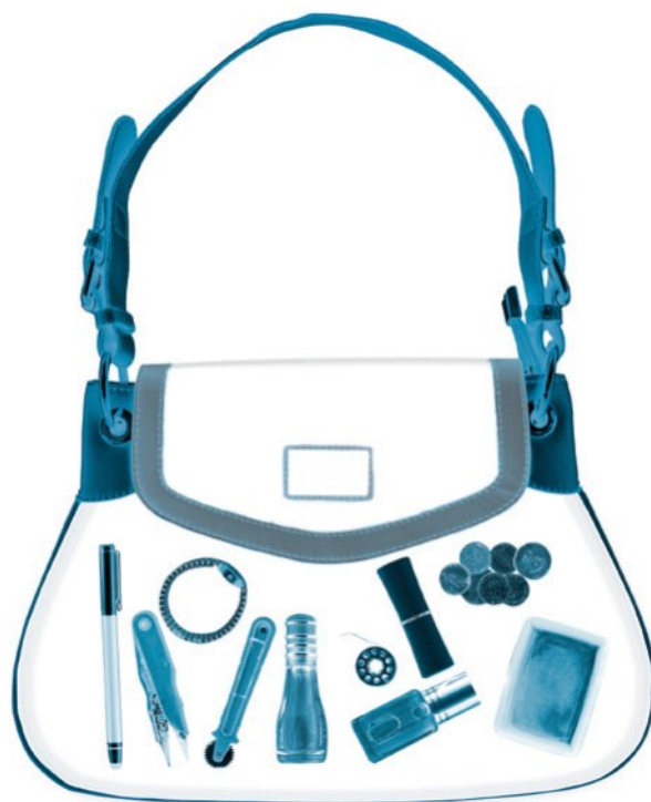
FIGURE 5.4.6 Variations in the density of luggage items mean that X-rays penetrate samples to different extents. Such variations are used to build an image.
