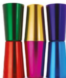
FIGURE 3.1.8 These cups are made of anodised aluminium. Their surface is a layer of aluminium oxide that was deliberately built up on the surface of the metal and then coloured.
