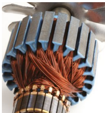
FIGURE 6.4.5 In an electric motor, current is passed through a coil. The magnetic field it produces interacts with the permanent magnetic field of the motor, causing the coil to spin.
