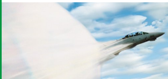
FIGURE 5.1.9 When an aircraft flies faster than the speed of sound it creates a shock wave like the one spectacularly shown in this photo.
