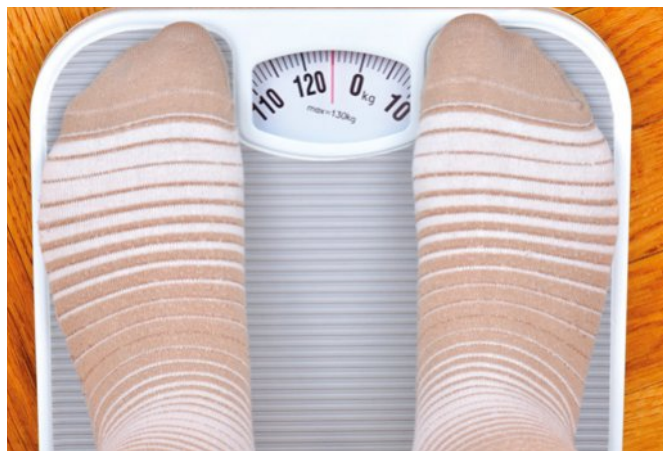
FIGURE 1.4.7 Before stepping onto bathroom scales they should read zero. A reading above or below zero will result in an incorrect reading called a systematic error.
