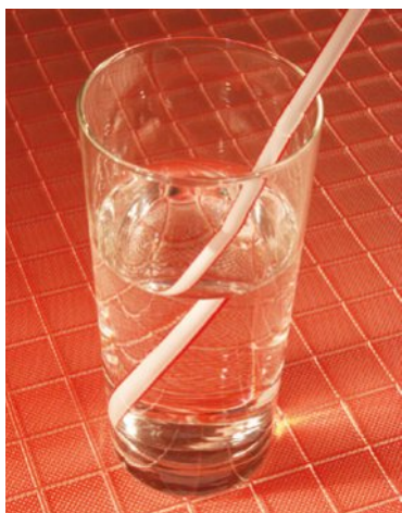
FIGURE 4.3.8 This straw appears disjuncted at the surface of the water, when viewed through the water in the glass.
