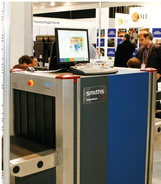
FIGURE 5.4.5 X-ray baggage inspection systems are widely used to screen luggage at airports.
