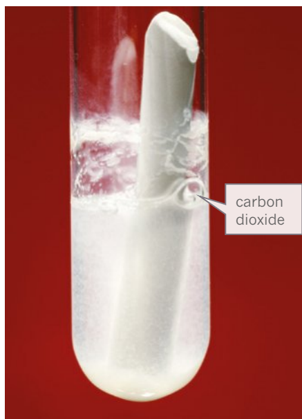
FIGURE 3.2.2 Chalk contains the base calcium carbonate. Here hydrochloric acid reacts with the calcium carbonate to form bubbles of carbon dioxide.
