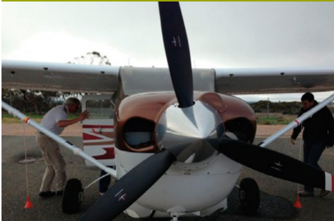
FIGURE 9.2.18 An aircraft used for counting kangaroos. The red weights and cord attached to the wing struts are used in the count.
