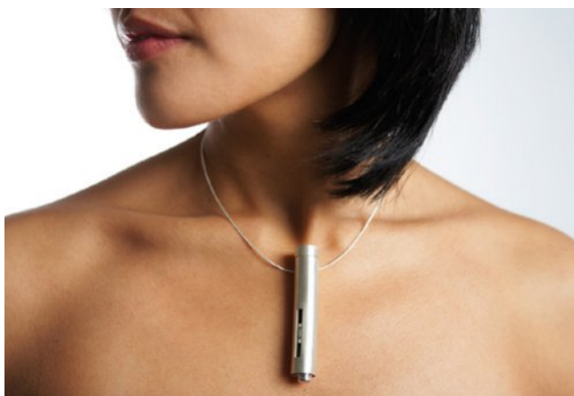
FIGURE 2.2.5 Diabetes jewellery designed by Leah Heiss. The Diabetes Neckpiece is an applicator device that applies small, circular discs covered in micro needles that deliver insulin through the skin.
