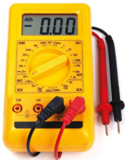
FIGURE 6.2.8 A multimeter combines an ammeter and a voltmeter, and can also measure resistance.
