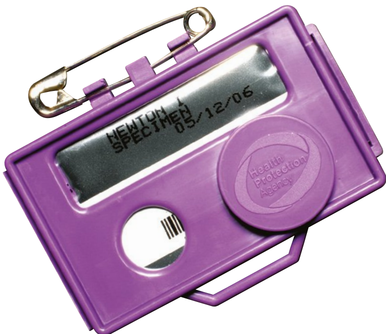
FIGURE 5.4.4 A personal radiation monitoring device measures a person's exposure to X-rays, and other forms of harmful radiation.
