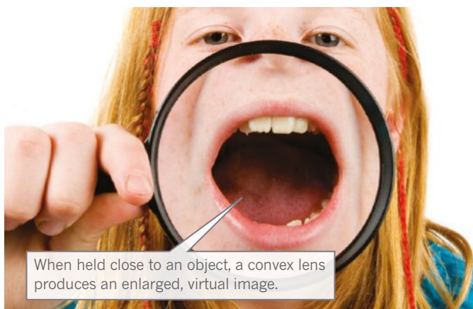
FIGURE 4.3.16 Lenses refract light to produce different types of images. A magnifying glass is a convex lens.
