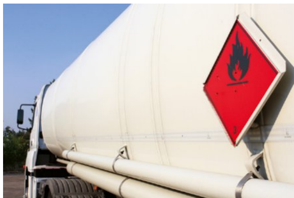
FIGURE 1.2.3 Trucks transporting hazardous substances, such as flammable liquids, must have hazard symbols attached.
