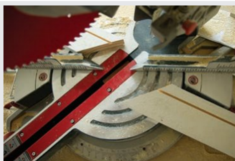
Carpenters use an electric Mitre Saw to make accurate cross cuts at any selected angle. Applications include making angled cuts for the corner joints in picture frames, door frames, architraves, skirting and cornices.
