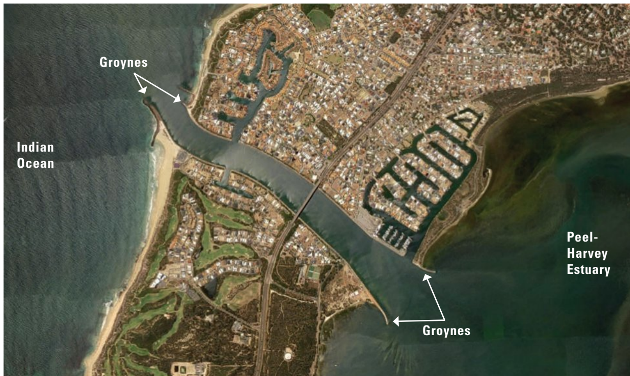
▲ Figure 6.41 Entrance to the Dawesville Channel. Can you explain why the groynes are designed in this way?
