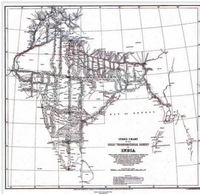
A map showing the triangles and transects used in the Great Trigonometric Survey of India, produced in 1870
