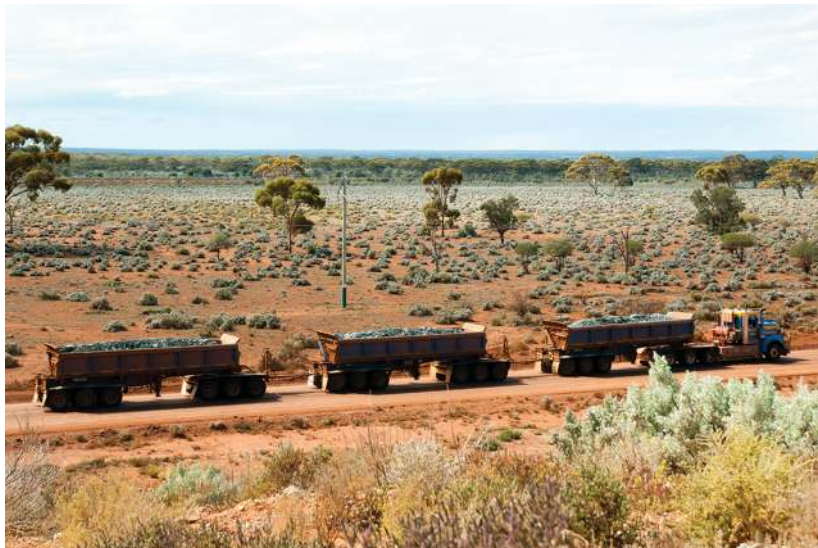
The average speed (85 km/h) of a road train and its capacity (120 tonnes) are used to schedule the delivery of mined ore to each ship when in port.
