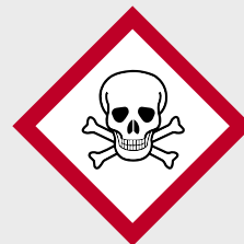
Figure 1.11 Skull and cross bones – toxic Can cause death if touched, inhaled or swallowed.
