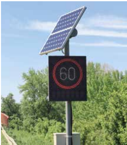
Figure 3.26 Solar-powered speed signs are becoming common all across our country and help save energy too.
