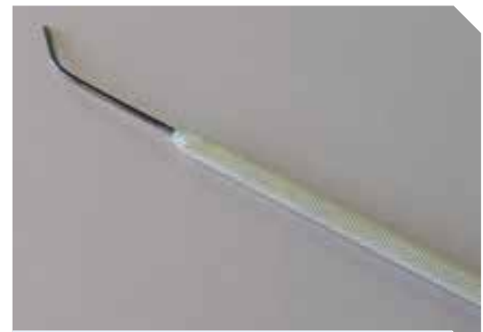
Figure 1.14 Probe Used to look at and explore a specimen, and to probe openings.
