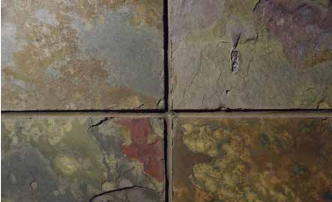
Figure 2.28 Slate cleaves easily into flat sheets because of its flat, parallel crystal structure. This makes it a useful material for floor and roof tiles and as the base for billiard tables.
