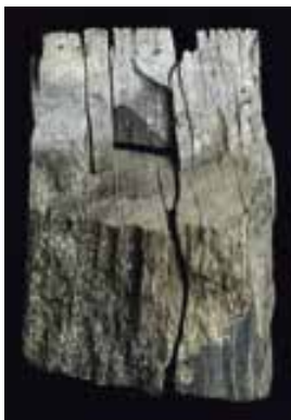
Figure 2.20 Shale (or mudstone) is the most common sedimentary rock. Shale is a fine-grained sedimentary rock made up of clay minerals or mud. This specimen clearly shows the layers of sediments that were compacted to form this rock.
