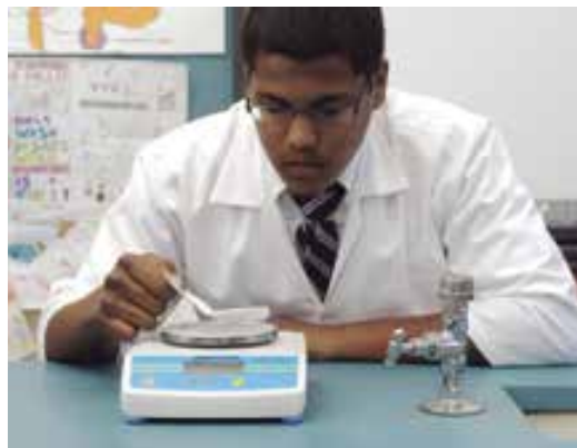
Figure 9.42 Weighing the eggshells allows you to calculate the mass lost in the reaction.
