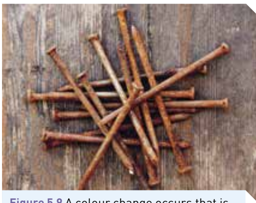
Figure 5.9 A colour change occurs that is non-reversible. Heating an iron nail to red hot is a physical change because the red colour will disappear as the nail cools down. However, if the iron in the nail reacts with air and becomes rusty, it is a chemical change.
