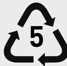
Figure 5.30 Polypropylene (PP) is used to make microwave meal trays, sauce bottles, yoghurt containers and medicine bottles.
