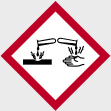
Figure 1.7 Corrosive Substances that are corrosive (destructive) to living tissues, such as skin and eyes. Also used for substances that are corrosive to metals.
