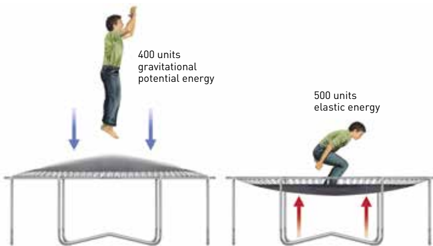
Figure 3.32 Five hundred units of energy are stored in the springs of the trampoline. At the highest point, the jumper has 400 units of gravitational potential energy. Where have the 100 ‘missing’ units gone?
