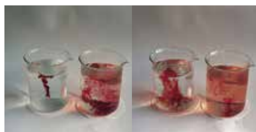
Figure 4.21 Diffusion occurs faster in hot water (right beaker) than in cold water (left beaker).
