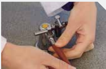
Figure 9.14 Connect the rubber hose firmly to the gas tap.
