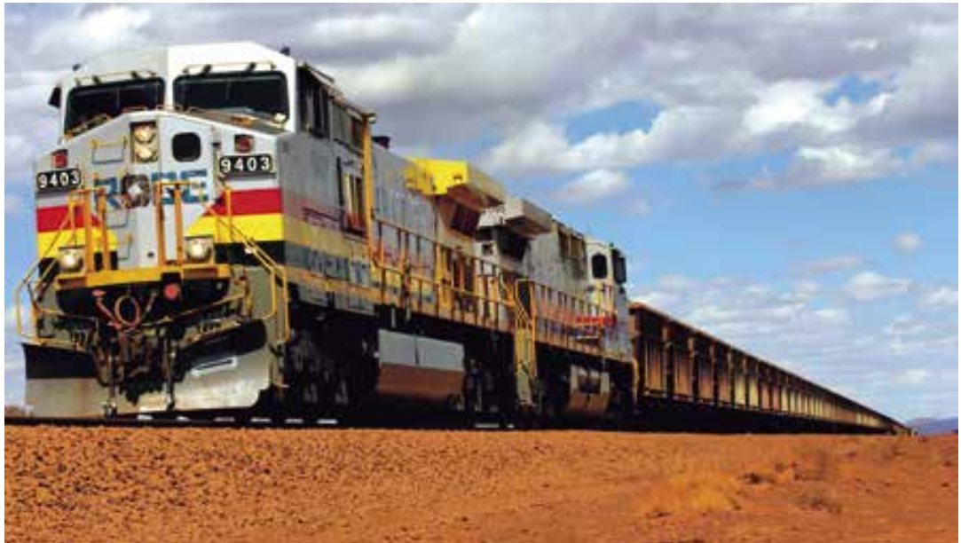
Figure 3.11 Powerlines aren't practical in rural areas, so diesel fuel is used.
