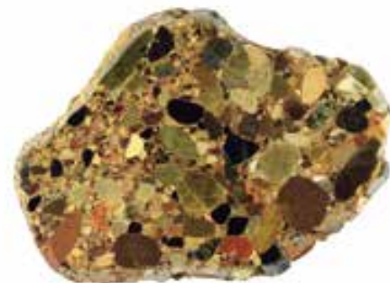
Figure 2.23 Conglomerate rocks have grains of different sizes. The sediments for these rocks were deposited in fast-flowing rivers during flooding or by glaciers.
