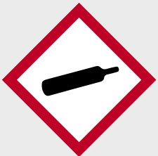
Figure 1.6 Gas cylinder Contains gas under pressure. Released gas may be very cold. Gas container may explode if heated.
