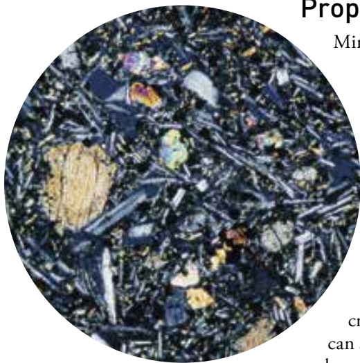
Figure 2.7 The individual mineral crystals of the rock olivine basalt can be seen under a microscope.
