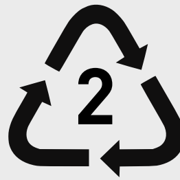
Figure 5.27 High-density polyethylene (HDPE) is used to make milk and juice bottles, some washing-up bottles, toys and grocery bags.
